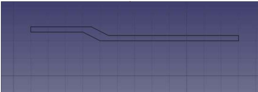
select multiple objects - and use the join tool. In the combo view, we will see the four segments disappear, to be replaced by a single Wire object.
