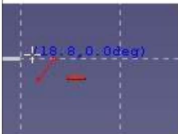
One vertex of a segment with a horizontal constraint
