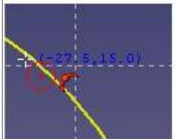
Snapping onto an arc
