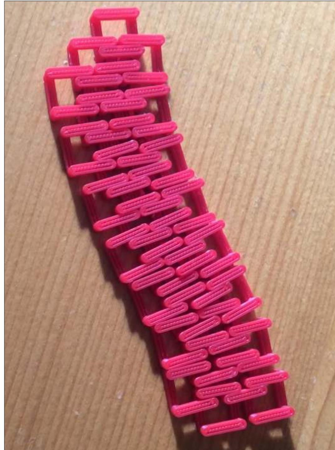
this direction, rounded links can be transformed into a collection of simple volumes (cylinders and bars), such as in the adjoining STL file (captured in Meshlab).
