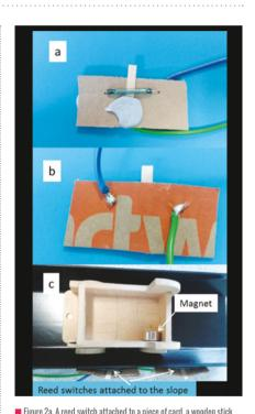
so its location is readily visible when in-situ and Blu Tack to attach the unit to the slope. b. Reverse side of image a showing the wires attached to the reed switch, c. A trolley fitted with a magnet and two reed switches attached to the slope
