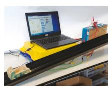
Figure 1. Finished experimental setup of a trolley on a slope attached to a Makey Makey and laptop running a Scratch program
