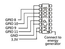
■ How to connect the ADC MCP3008 to the Raspberry Pi
