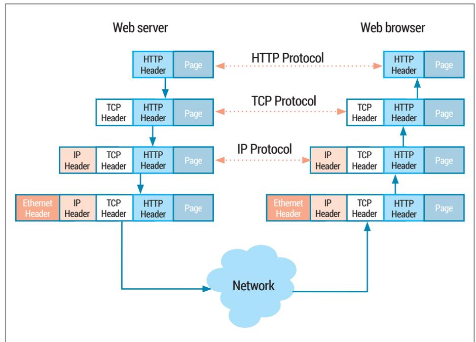
Figure 1: As a packet passes down through the layers of a protocol stack, each layer’s header forms part of the payload of the layer below.
