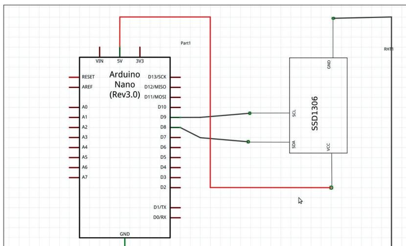
The fritzing diagram showing the connections for an Arduino Nano. It is straightforward though – just direct connections for the power and the two pins we use for I2C (in this case D8 and D9).
