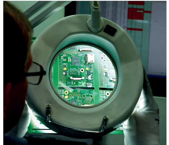
top of the Raspberry Pi, with special attention being paid to the BCM2835 processor unit, which requires a memory chip to be installed on top of it using a specialist package-on-package (or PoP) applicator that adds a small amount of solder paste to the balls of solder on the bottom of the memory chip; this is then lowered onto the BCM2835 to make the connections.
