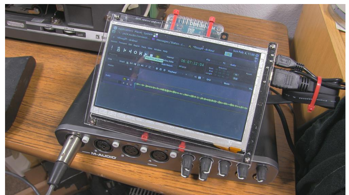
Figure 1 – An ODROID-XU4Q recording voice-over via USB interface
