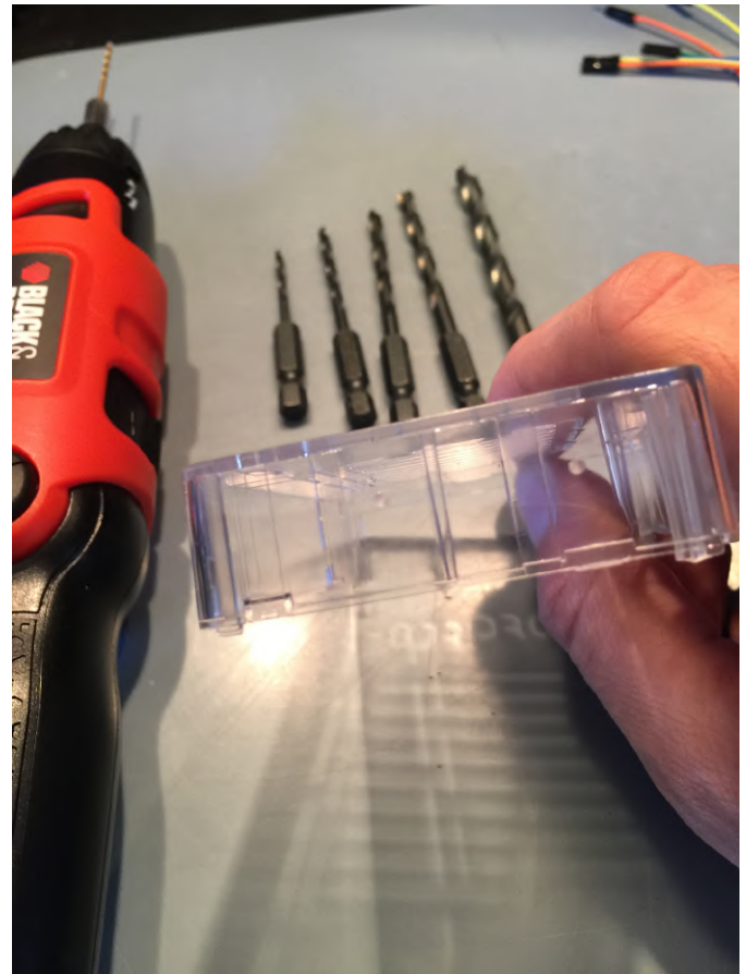
Figure 4 - Drill through the paper into the plastic, just deep enough to leave a bit of a visible mark
