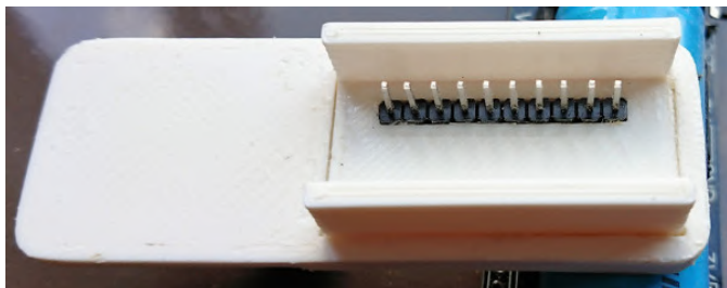
Figure 3 : A photo of the back of the enclosure showing the header pins glued in
