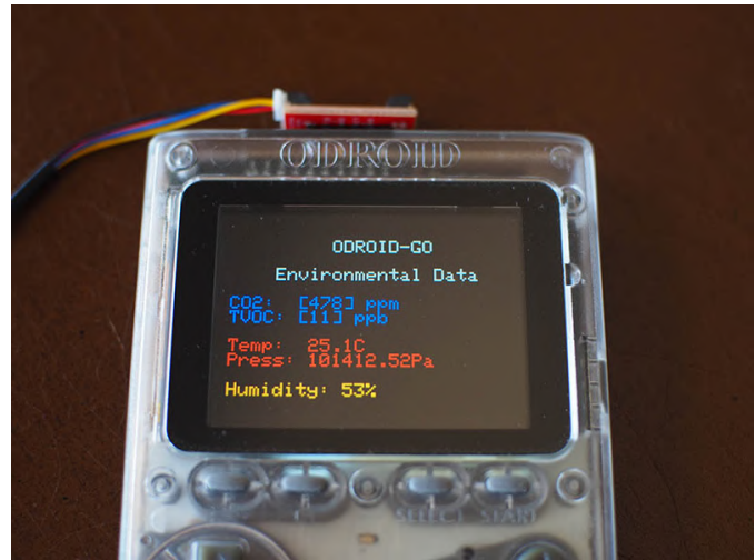
Figure 3 - A sample output from the Qwiic Environmental Combo Breakout.
