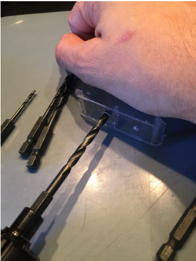
Figures 5 and 6 - Each run-through with a bigger drill bit creates a slightly larger hole
