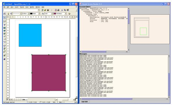
Illustration 18.1: The simple screen reader shows information on the currently focused object in two different views. A textual display on the top left shows its description, states and bounding box as well as the names of its ancestors. The graphical view on the top right shows the bounding boxes of the object itself (green) and its ancestors (gray). The bottom window logs all events sent by any of the accessibility objects.
