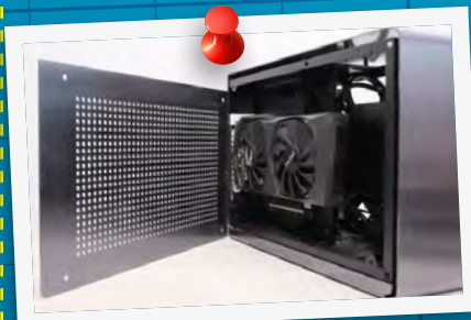
A mini-ITX case with a large vented side panel can outperform the cooling of some ATX cases
