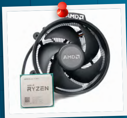
The cooler supplied with some CPUs will handle your CPU at stock speed, but not overclocked
