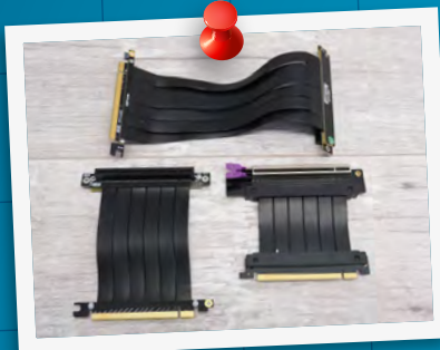
PCI-E 3 riser cables supplied by case manufacturers can cause serious stability issues with a PCI-E 4 graphics card and motherboard
