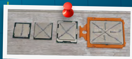
For the best results, apply thermal paste in different shapes depending on the size of your CPU's heatspreader
