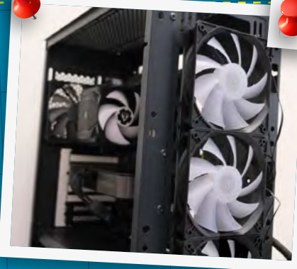
We recommend having one front fan in line with your CPU and another one in line with your graphics card
