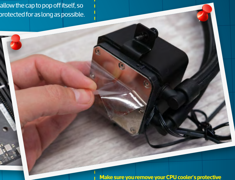
Make sure you remove your CPU cooler's protective cover before fitting it
