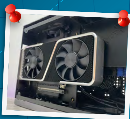
Placing your graphics card right next to an unvented side panel seriously impacts airflow
