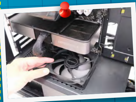
Pointing a fan directly at your graphics card from below can help if it has a flow-through cooler design
