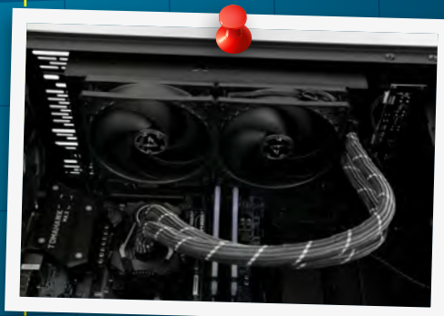
The roof of your case is the best location for a liquid cooler's radiator
