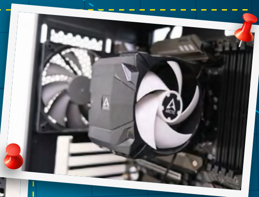
Always point your CPU air cooler in the same direction as the rear fan
