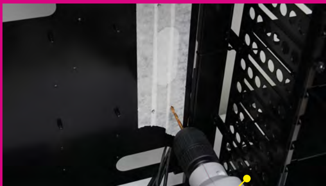
Use a drill on a medium speed setting to create the holes
