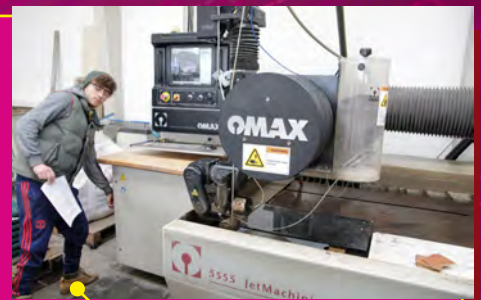
We turned to a local water jet cutting service to get some vents cut into a case
