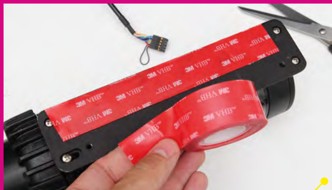
As long as your component has a large mounting plate, 3M mounting tape is strong enough to hold it in place
