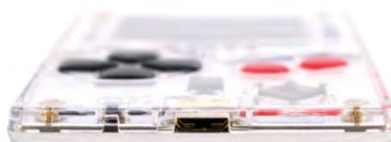
As with the original Arduboy, power and data connect over a micro-USB port
