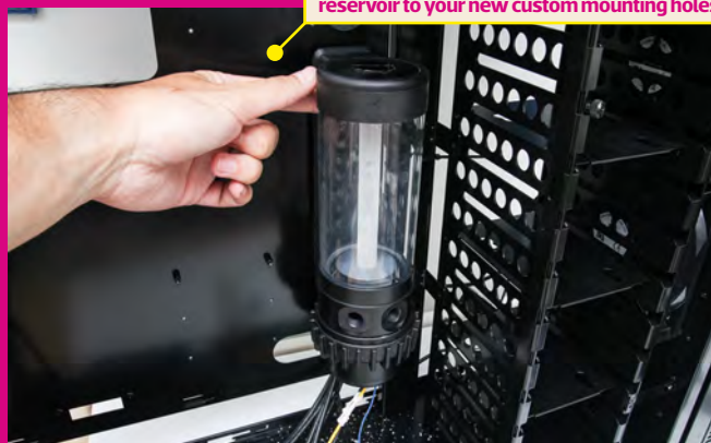
Use the included screws to secure your reservoir to your new custom mounting holes
