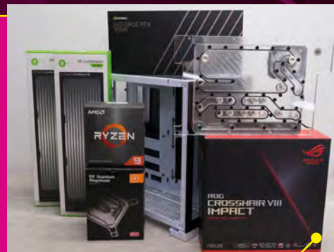
We're using a distro plate in our water-cooling loop, rather than a standard reservoir/pump unit
