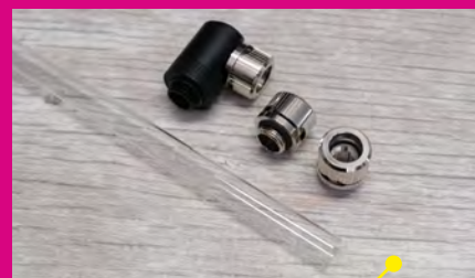
You can use angled fittings to avoid having to bend your rigid tubing at certain angles
