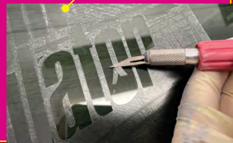
We used a vinyl cutter to create a mask for the etching cream
