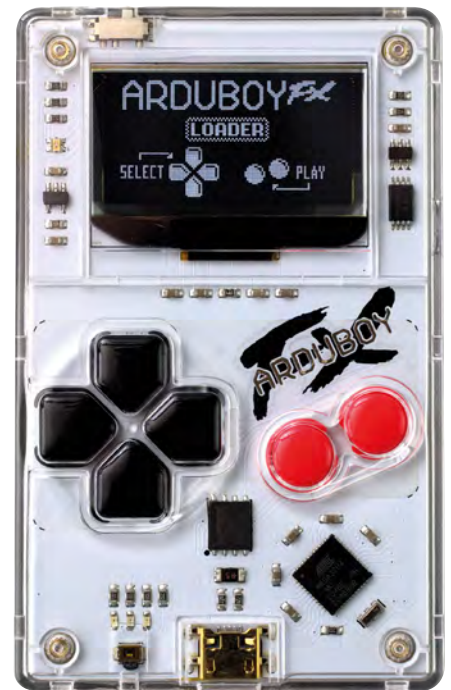
The Arduboy FX is near identical to its predecessor, bar a new flash chip
