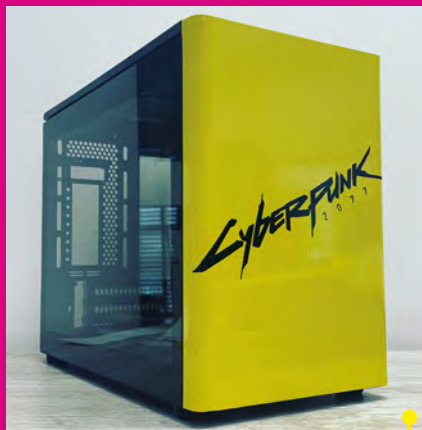
You can place the vinyl on paint or on top of other vinyl, such as this black vinyl on top of a yellow vinyl wrap
