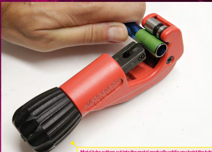
Metal tube cutters cut into the metal gradually while you twist the tube
