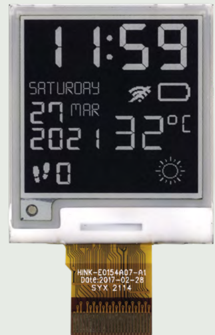
The e-paper display needs power only when changing states, and is fully readable in sunlight
