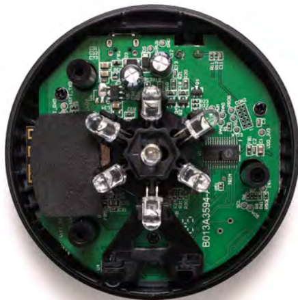
The 'hedgehog' array of IR LEDs provides broad coverage for signal transmission
