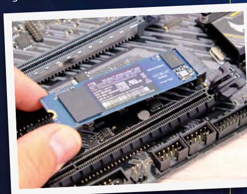
Every M.2 SSD you use instead of a SATA drive saves two cables from cluttering the inside of your case
