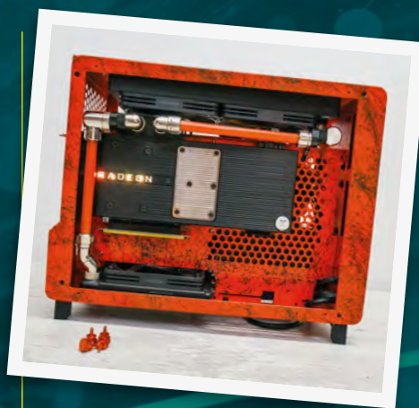
Sandwich cases, which mount the motherboard in the middle, aren't great for air cooling but they're often good contenders for water cooling
