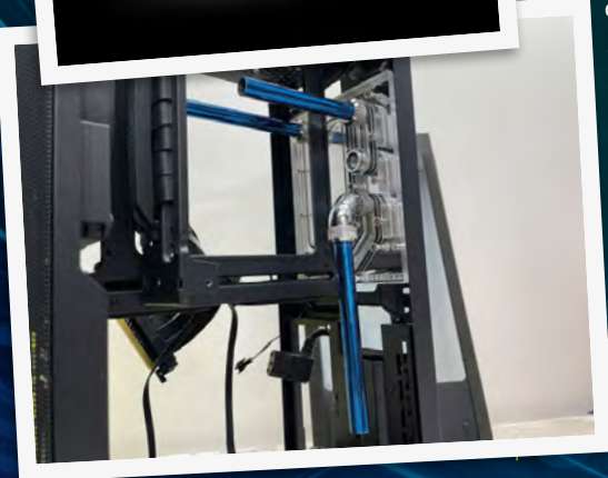
Phanteks' Glacier D120 distro plate can be mounted on a flat surface or in a 120mm fan mount
