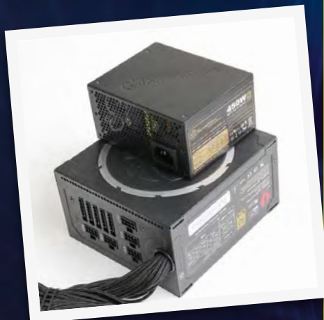
SFX PSUs are smaller than ATX PSUs in every dimension
