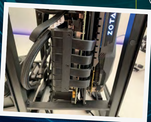
PCI-E risers enable your graphics card to sit in different positions and not be directly attached to the motherboard
