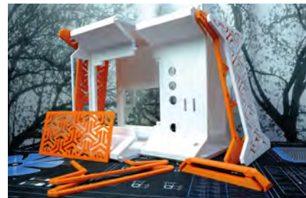
Almost all of the non-component parts of the build are 3D printed
