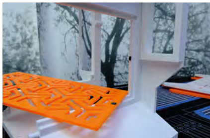
Magnets were used to attach the front and side grilles to help with accessing the case
