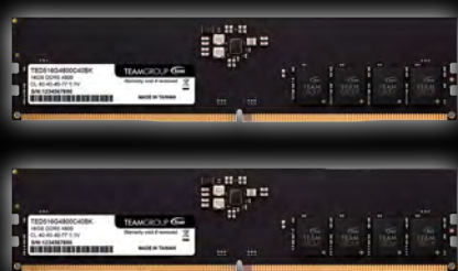
A cluster of power management circuitry is now a prominent feature on most uncovered DDR5 DIMMs
