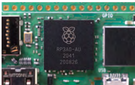
This chip packs the SoC and 512MB of RAM in two dies
