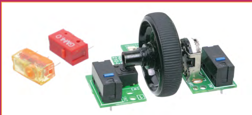
The left, right and scroll wheel switches can all be replaced, along with the scroll wheel encoder
