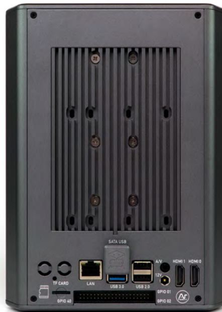
The rear includes full-sized HDMI ports and two break-outs for an as yet unpopulated expansion header
