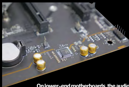
On lower-end motherboards, the audio codec tends to be left uncovered
