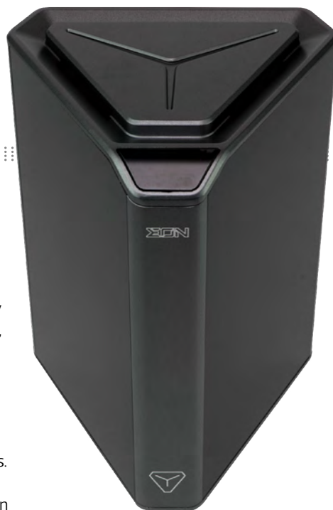
The big sibling to the Argon One, the Eon packs in up to four SATA drives for a home-brew NAS system
