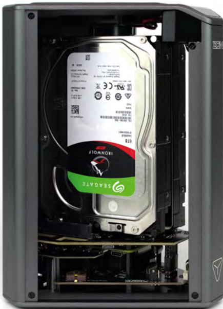
For best results, use 2.5in drives; you can squeeze two 3.5in drives into the Eon, but they practically end up touching
