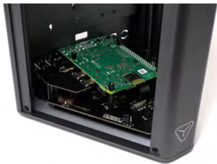
The Raspberry Pi 4 mounts upside down, with pillars connecting to the system-on-chip and RAM for cooling
