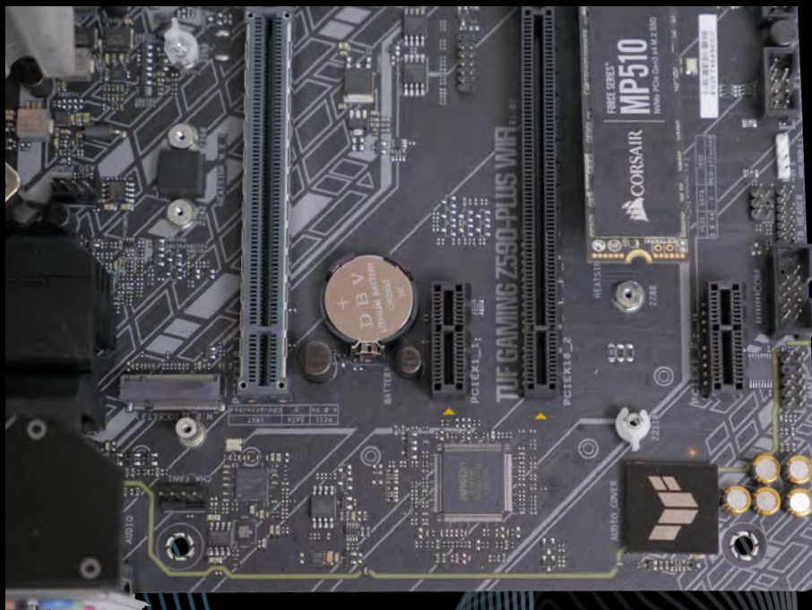
On higher-end motherboards, the audio codec is often shielded from interference by an extra cover
