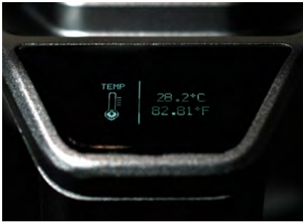
The OLED display is handy, although it fails if you configure a slow fan speed
