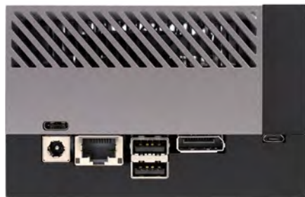
The SOM has capacity for four 10Gbps Ethernet ports, plus a Gigabit port, but only a single 10Gbps port is broken out
