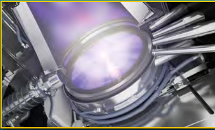
An ASML EUV source vessel, where a powerful laser hits tin droplets to generate extreme ultraviolet light
