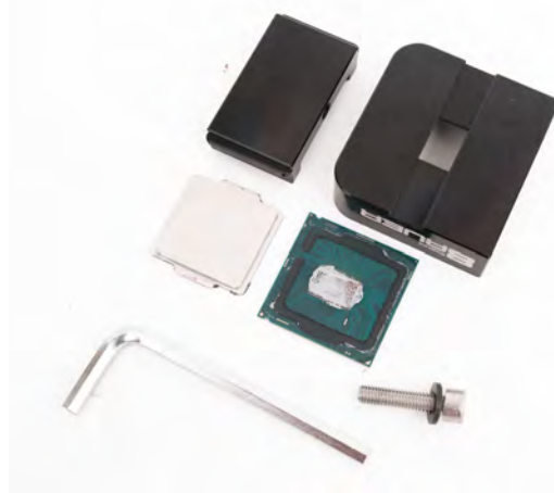
A delidded CPU, courtesy of a De8auer kit
