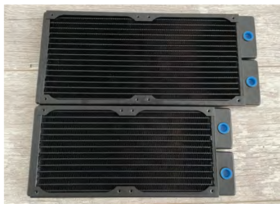
Alphacool's slim radiators are available in 140mm variations, which offer much greater surface areas than their 120mm equivalents
