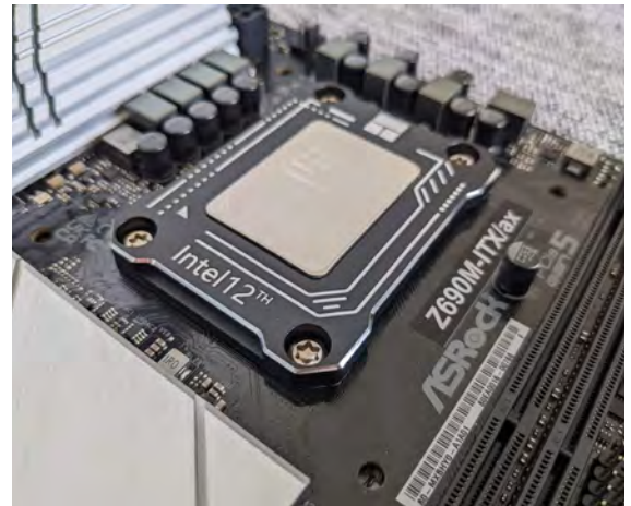
You can use a support bracket to prevent LGA1700 CPUs from bending
