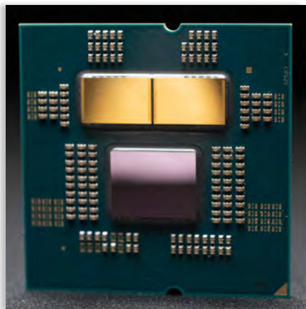
Each Ryzen 7000-series chip will include one IOD die (centre) and one or two CCDs (top left and right)
