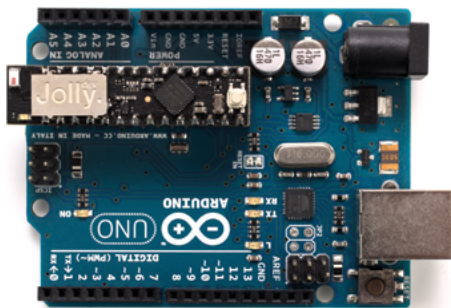
The module fits where the ATmega328P chip would usually sit, although it stands proud of the headers
