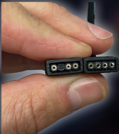
On the left is a 5V 3-pin RGB connector. The fourth hole is blocked, which means it's impossible to connect it to a 12V 4-pin header
