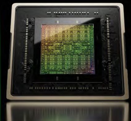
The AD102 is manufactured using TSMC's latest 4N (5nm) process, more than doubling the density of its previous chips
