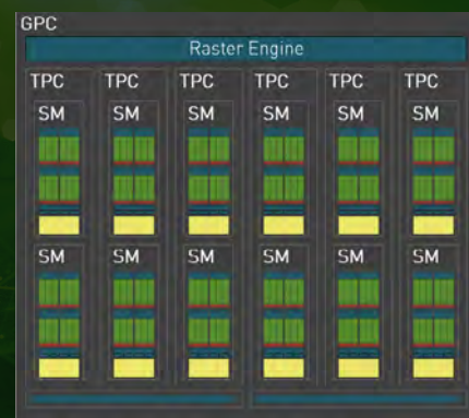
The GPC of AD102 is structurally identical to that of the Ampere architecture
