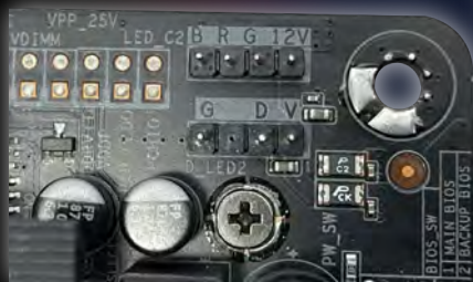
Most motherboards are equipped with both 12V 4-pin and 5V 3-pin headers to control both types of lighting
