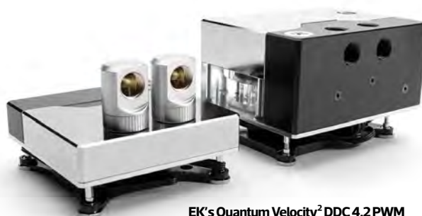
EK's Quantum Velocity 2 DDC 4.2 PWM D-RGB (right) stands only a little taller than a waterblock with barbs, but there's a waterblock, pump and reservoir inside
