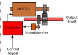
The control signals are expected in a very specific "format", and we will use PWM (Pulse Width Modulation) for that. First, the pulses must come every 20 milliseconds. The width of the pulse determines where the output shaft turns to. If the pulse is 1 ms in width, the motor will move toward 0°. If the pulse is 1.5 ms, then the shaft moves toward 90°. If the pulse is 2 ms, the shaft moves toward 180°
