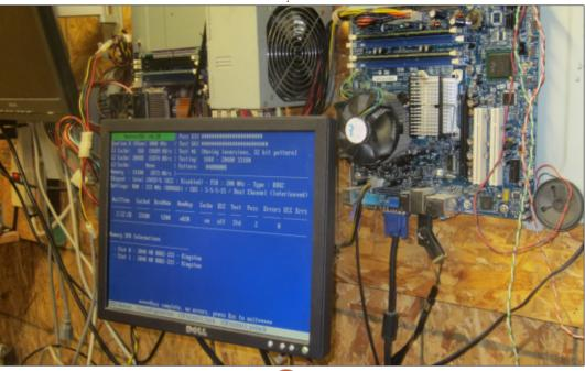
Across from the small item ewaste wall is a workbench that's used for a number of functions: memory testing, soldering, and cleaning computers. Three motherboards are screwed into the wall. We boot Memtest86+ from USB key on each of these boards to test RAM covering SD-RAM, DDR, DDR2 and DDR3. On the odd occasion we get RAMBUS RIMM RAM we usually test the RAM in the machine the RAM originally came in. This is also the case for "Registered" and "ECC" RAM.
