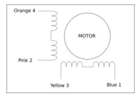
The numbers shown with the colors of the wires are for the 28BJY and yours may be different. The wire connector (if there is one) might differ from unit to unit. You can use an ohmmeter to verify the coils.
