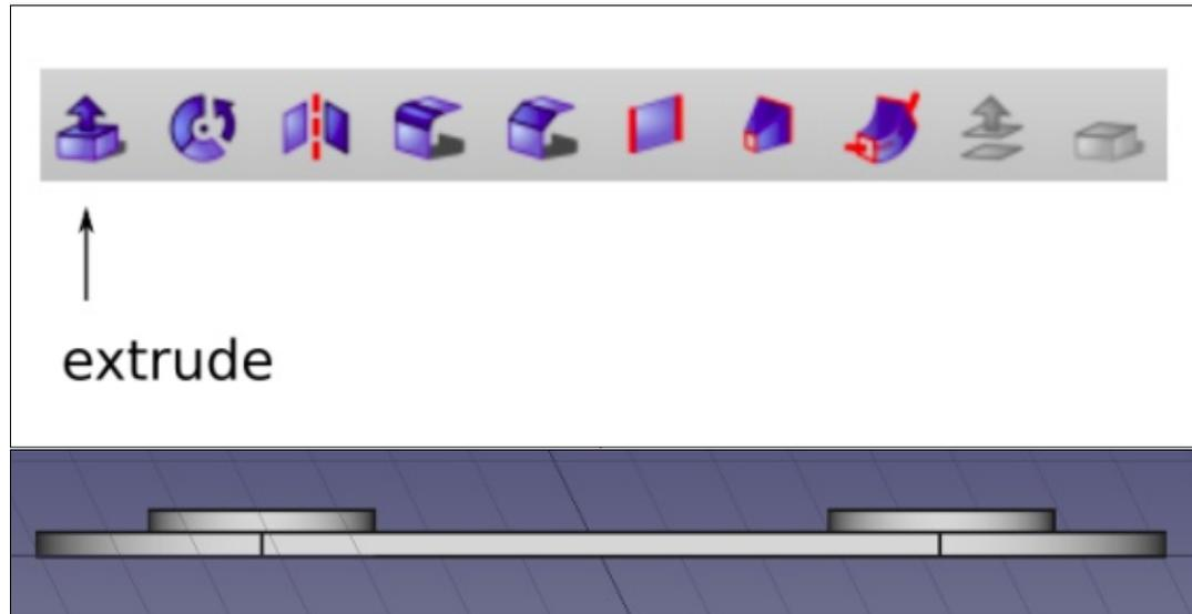
Now do the same with the other circle, converting it also into a cylinder 4 mm high. Finally, let us make an extrusion from the Wire piece, but this time only 2 mm high.
