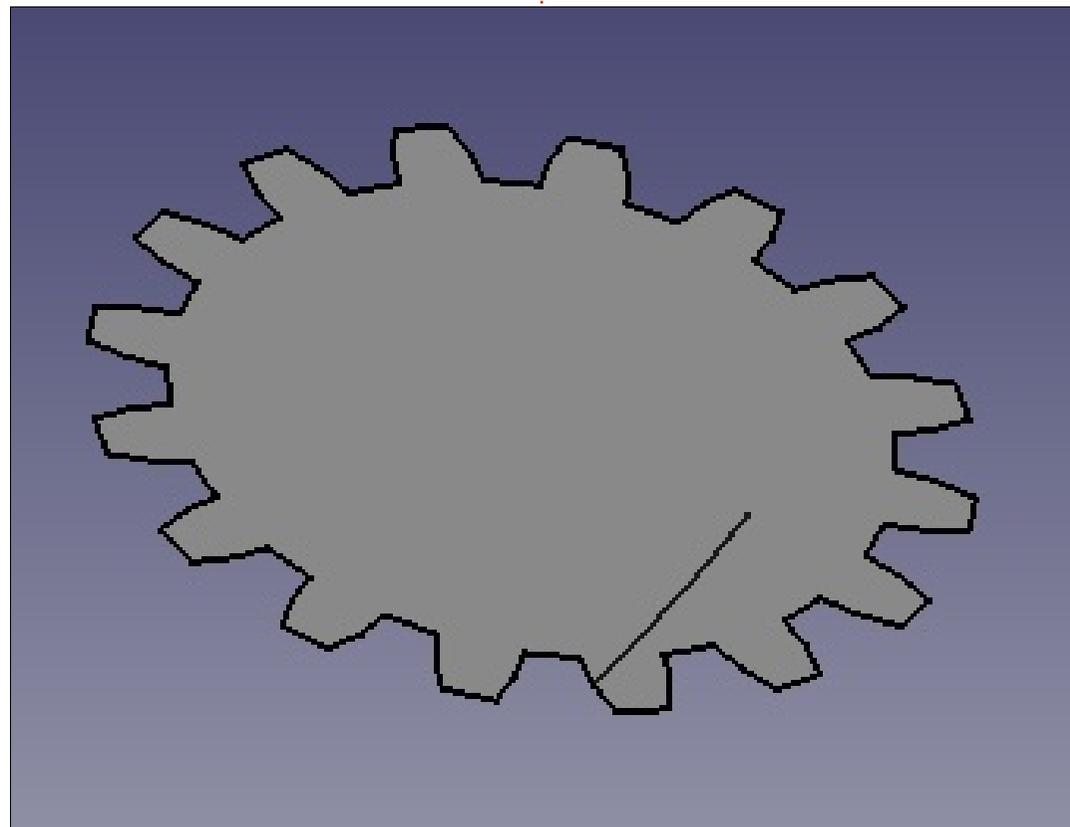
approximately 1:20 across the width of the wheel, I chose a helix height of 50 mm, but a pitch of 1000 mm between helix spires. The external radius of the helix should correspond to the point at which it will be created. Both right-handed and left-handed helices can be used, as needed.
