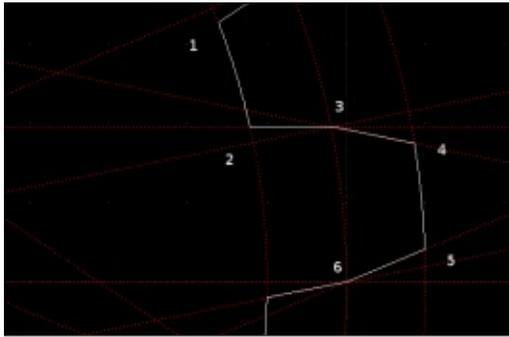
and 5 are on this radius, in our case taken at 110 mm. Finally, we need to “make some space” inwards, to accommodate the other wheel’s teeth. So we go inwards to the bottom flat, at radius 90 mm in our case, and holding points 1 and 2. We will iterate this basic shape over the 16 teeth of our wheel.
