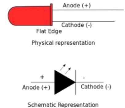
LED on, so we’ll connect the 220 ohm resistor directly between the 3.3 volt pin and the Anode of the LED, then connect the Cathode to our GPIO pin to complete the circuit. For the switch, we’ll connect one side of the switch directly to ground and the other directly to a different GPIO pin
