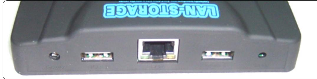
the PCs without needing to share folders on the PCs, and allows them to be powered and accessible all the time. The only downside to using this low-power server is, the network speed is quite LOW. (1Mb/s write and 2Mb/s reading) - however the speed is sufficient to stream 720p movies to my media
