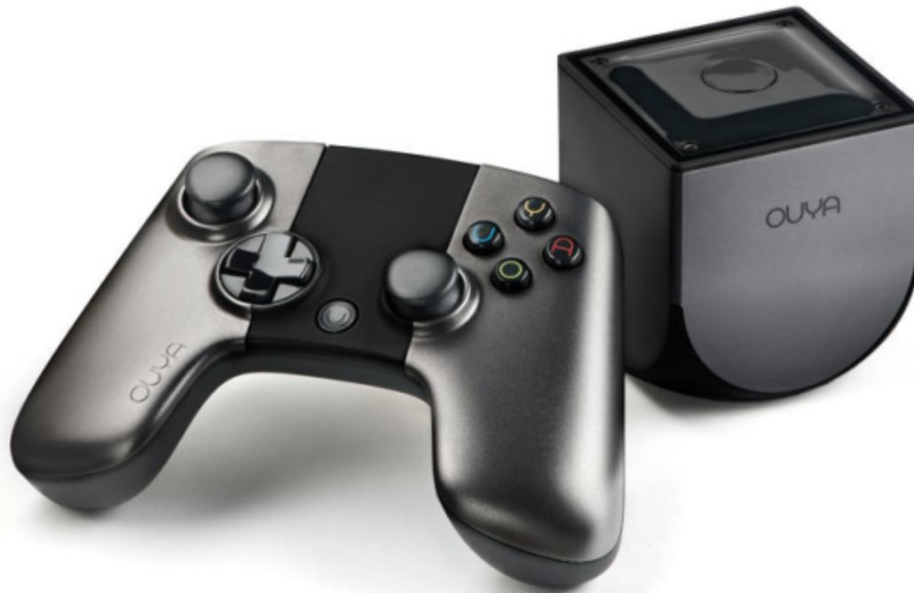
wireless, has a small touchpad (above and between the d-pad and right stick), and is about the size of your average Playstation/Xbox controller, but not as heavy. It has the usual array of buttons (four), two sticks, one d-pad, and four shoulder buttons. Between the d-pad and right stick is the Ouya button.
