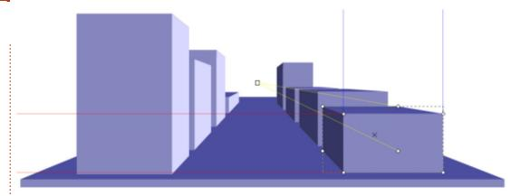
Returning to a single box, let's try some 2-point perspective. Draw a new box if you need to, but this time, toggle the parallel lines buttons for both the X-axis and the Z-axis. Leave the Y-axis with an infinite VP at an angle of 90°.
