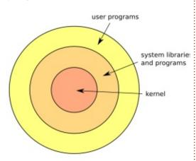
It is important to understand the purpose of each layer. The kernel itself is a very low-level piece of software; that is to say, it is in immediate relationship with the hardware and manages the most basic functionalities of the operating system. These include:
