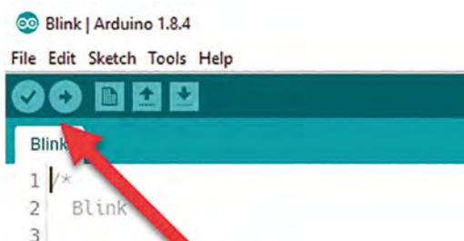
the upload process completes, the Arduino device will immediately reset, then begin executing the new sketch. In this example, the Arduino will turn its on-board LED on and off repeatedly until power is removed from the board or a different sketch is uploaded.
