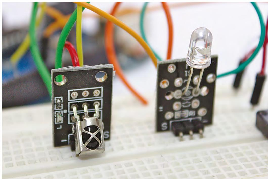
**Left** ◆ The receiver and the transmitter require only power and ground alongside a single data connection each to the Arduino
