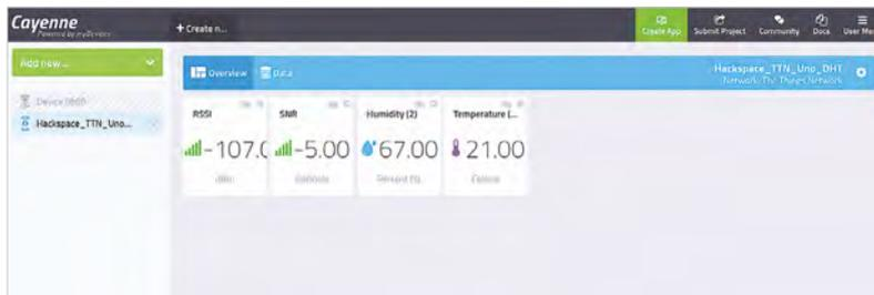
Our payload is decoded and is nicely displayed, labelled correctly 'temperature' and 'humidity', instead of just a raw collection of bytes
