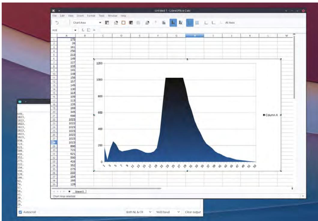
**Left** ♦ Generating CSV data from your sensors is a brilliant way to conduct experiments and visualise the output, such as the response curve from a piezo knock sensor
