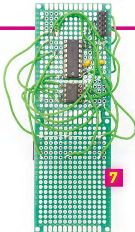
**Above** ♦ We found it easier to push the capacitors through from the side with the sockets and chips
