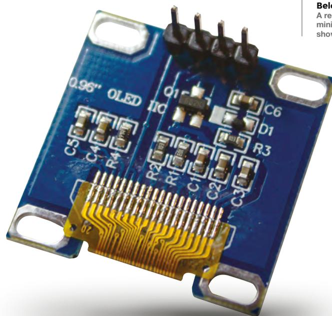
**Below** □ A rear view of the mini OLED display, showing its four pins
