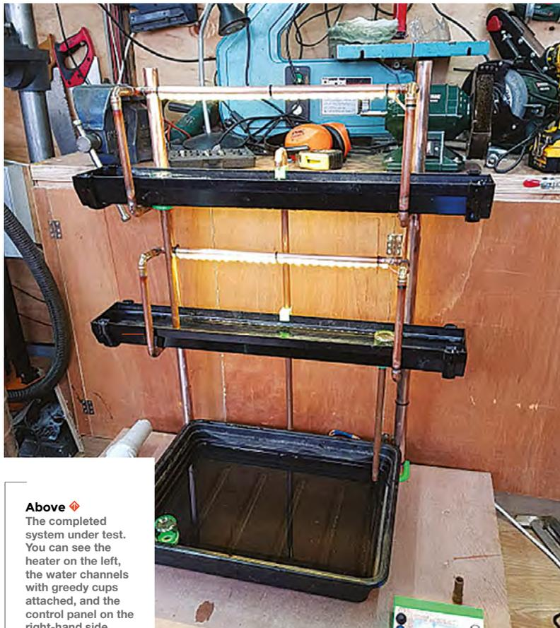
**Above** ♦ The completed system under test. You can see the heater on the left, the water channels with greasy cups attached, and the control panel on the right-hand side
