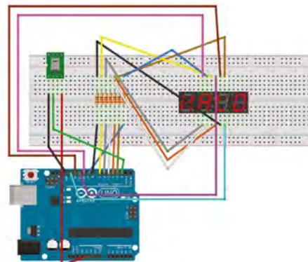
**Above** See the temperature and humidity changes in real time on your seven-segment display
