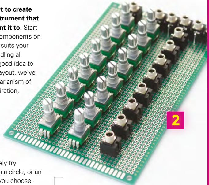
**Above** Start by playing with the component layout, without soldering anything
