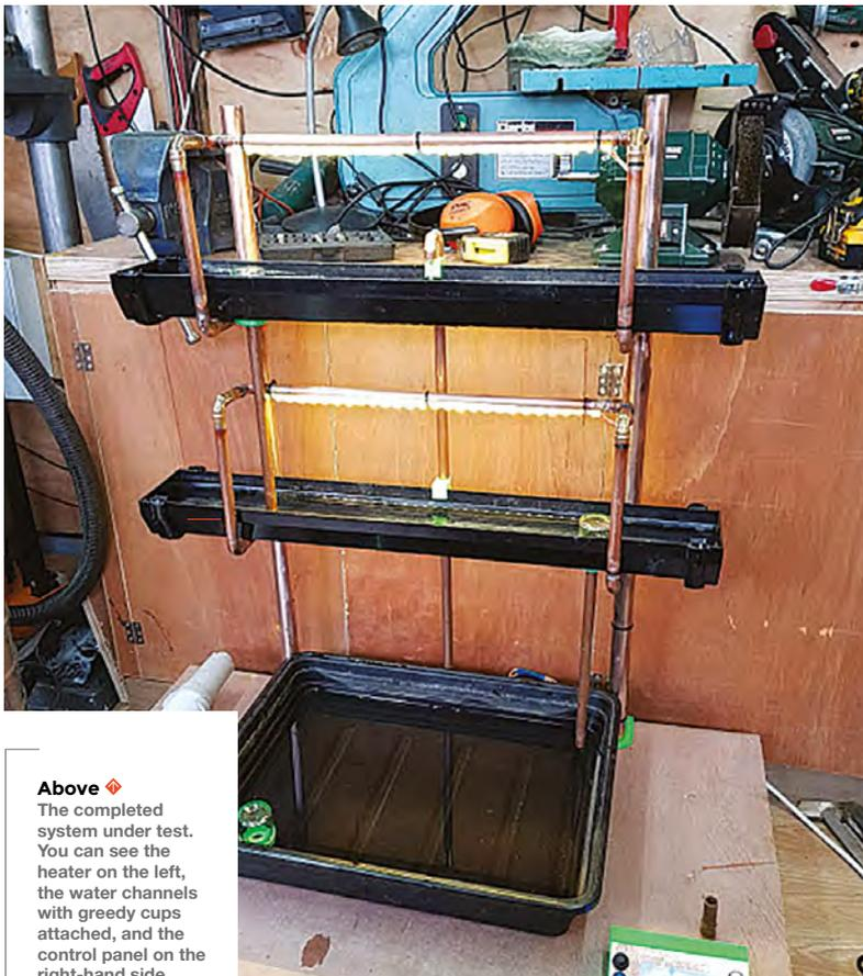
**Above** ♦ The completed system under test. You can see the heater on the left, the water channels with greedy cups attached, and the control panel on the right-hand side
