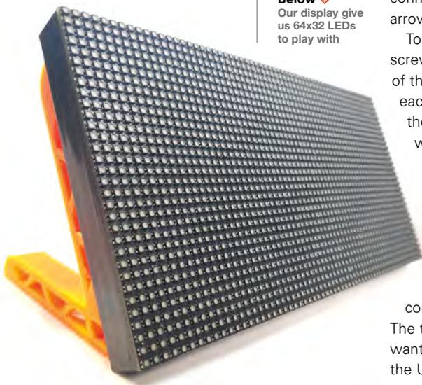
will have 64 LEDs across, and 32 LEDs down. This project is coded to work on 64x32 displays, but it could be adapted for other ones if needed.
