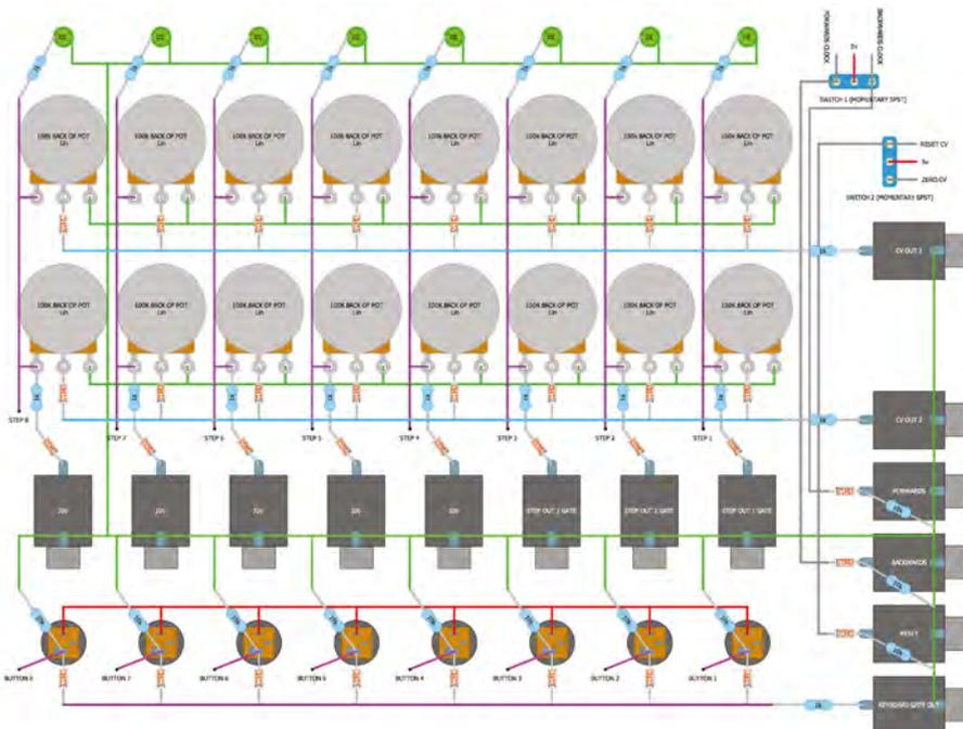
**Figure 1** ← This is what we're going to build – a sequencer for outputting voltages and an oscillator (VCO) for turning those voltages into notes
