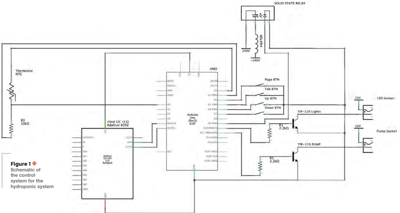
**Figure 1** ♦ Schematic of the control system for the hydroponic system
