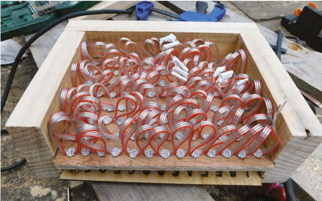
**Left** ♦ The LED string inserted. We had to join three strings together to get 104 LEDs for the clock. In hindsight, only 100 are needed, as some letters are never lit
