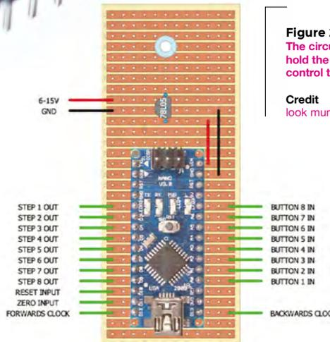
**Figure 2** The circuit layout to hold the Arduino and control the sequencer
