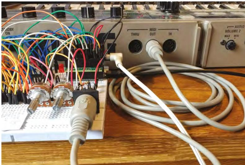
**Above** ♦ Many MIDI devices have three ports: 'in', 'out', and 'thru' – make sure to connect the MIDI out port of your external device to the MIDI in port on the breadboard
