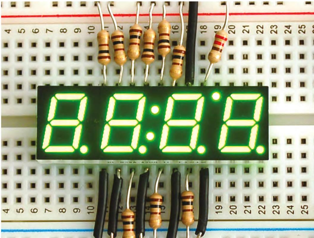
**Left** Multiple seven-segment displays may be multiplexed, and this allows them to run on fewer pins at the expense of more complex code
