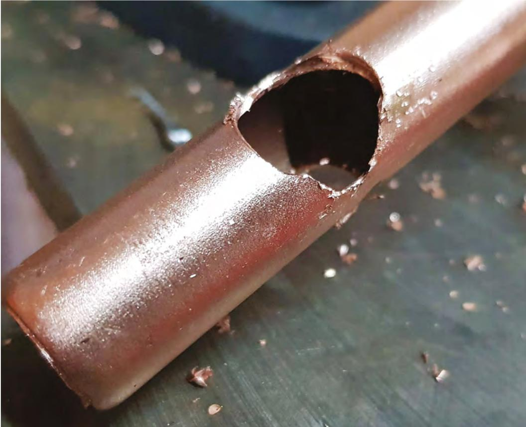
hole through the pipes, 750 mm from the end. The 15 mm pipe should slide through the hole in the 28 mm pipe and make a rudimentary shelf bracket. To figure out the length of the shelf brackets, measure the width of your guttering and add about
