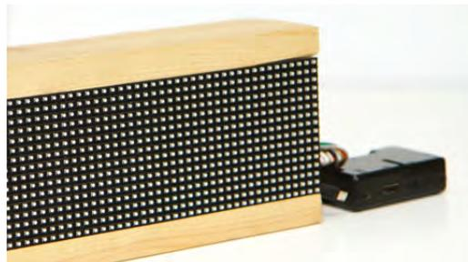
and reduce the brightness), you can use a reflective diffuser from an old broken LED TV if you can lay your hands on one from eBay or a TV repair shop, or just any other bit of translucent material. I found that two layers stapled on worked and looked great. Add some hooks to the back and – Bob's your uncle – a finished, wall-mounted display!
