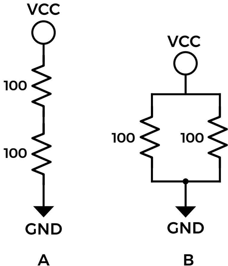
We'll use 5V for  $V_{cc}$ . What is the total resistance between  $V_{cc}$  and  $GND$  in each circuit? How much current is flowing through each circuit? What is the voltage across each resistor?
