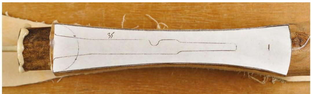
**Right** ♦ A scrap of sacrificial 3 mm ply and hot glue hold a 'round' wood blank in position for cutting
