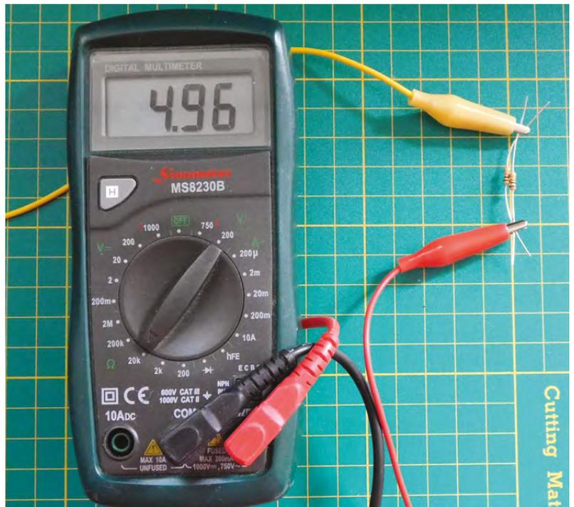
**Above** ♦ Two 10kΩ resistors in parallel read (almost) 5kΩ
