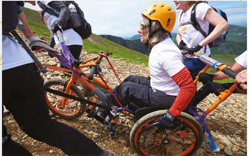
Fred, a retired engineer, looked at the possibility of using a bicycle frame as a removable front wheel for safely steering, braking, and lifting the wheelchair during the challenge. After numerous experiments, a modified BMX bicycle frame was securely fastened to Rosie's wheelchair with U-bolts and pipe clamps, enabling the Women of Altitude team to assemble and disassemble the wheelchair attachment during training sessions quickly. A lifting
