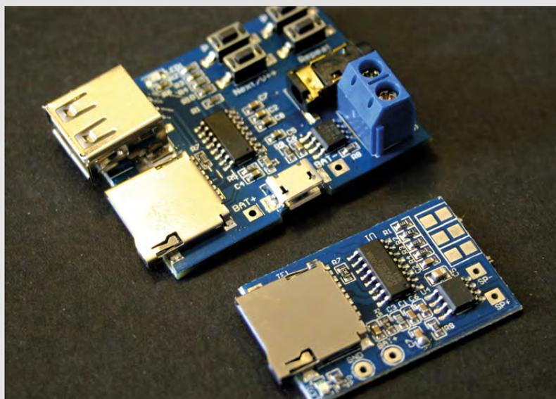
provides flexibility in the field, as does the ability to connect a battery. It just would have been nice to have a JST connector for lithium batteries to connect to, but at this price that would be asking too much. The speaker terminals are handy to have but, in all honesty, 90% of us will just connect an amplified 3.5mm speaker, so we could desolder those terminals to lower the height of the board, and of course add the terminals to our bits box.
