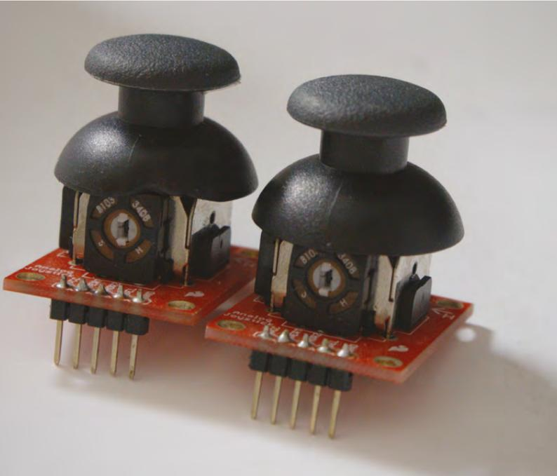
**Above** Soldering the joysticks to breakout boards will simplify your prototyping
