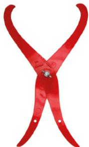
**Calipers are the ideal tool for checking the inner and outer dimensions of your piece.** This is especially critical for establishing symmetry and making sure different parts come together correctly. Use them to fit a lid to a pot, or a cup to the depression in a saucer. Once you have measured the width, tighten the caliper to secure the dimension for later use.
