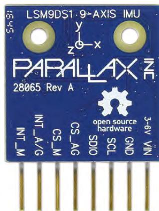
almost any microcontroller, and it can be powered by 2.8, 3.3, or 5 volts. Communication works with either a 3-pin SPI interface or an I<sup>2</sup>C bus, and features an interrupt which can be used for detecting and reacting to free falls or other inputs. It's all ready to use with the BlocklyProp environment, but you can use it with almost any other development environment too. □
