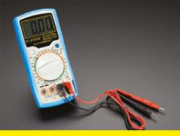
**Easy-to-use and affordable, a multimeter will be essential to measuring the fundamental parameters in electronics: voltage, current, resistance.** It will usually come with two probes: plug the black probe into the ground (COM) port,
