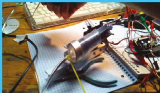
photos and videos. His universal gripper can pick up very irregular or smooth objects easily, despite the fact that it uses off-the-shelf syringes instead of expensive vacuum pumps and reservoirs. ▣
