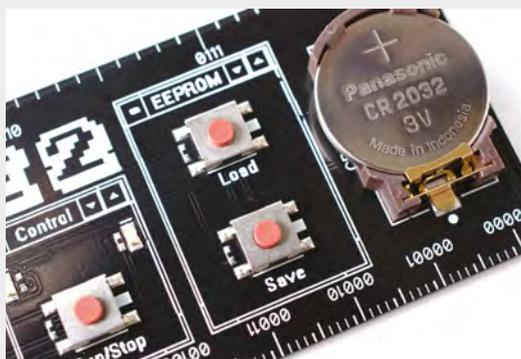
inserting binary bits – the zeroes and ones that are the only things a binary computer understands – into memory using the push-button switches. Each switch corresponds to one bit of an 8-byte memory address; a program can take up 256 bytes of memory in total, and there are eight slots for you to save programs into for later recall.
