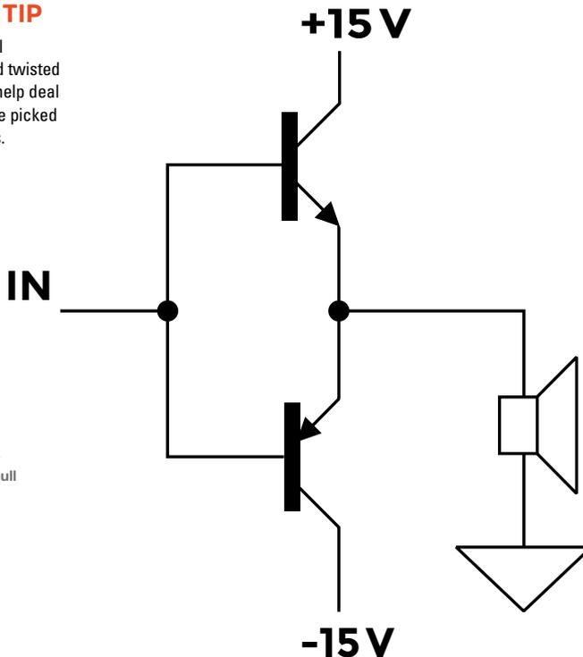
Figure 10 Basic push-pull amplifier
