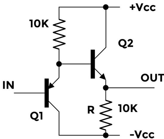
output has to be AC-coupled as well to remove the DC bias and pass the AC signal through.
