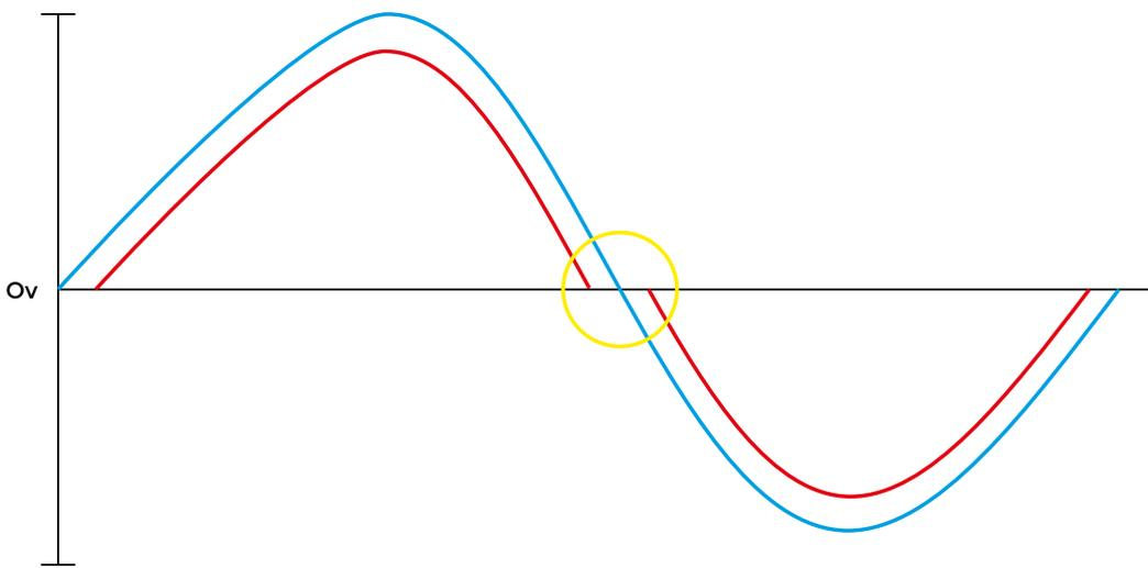
**Figure 11** Input vs. output in a naive push-pull amplifier circuit
