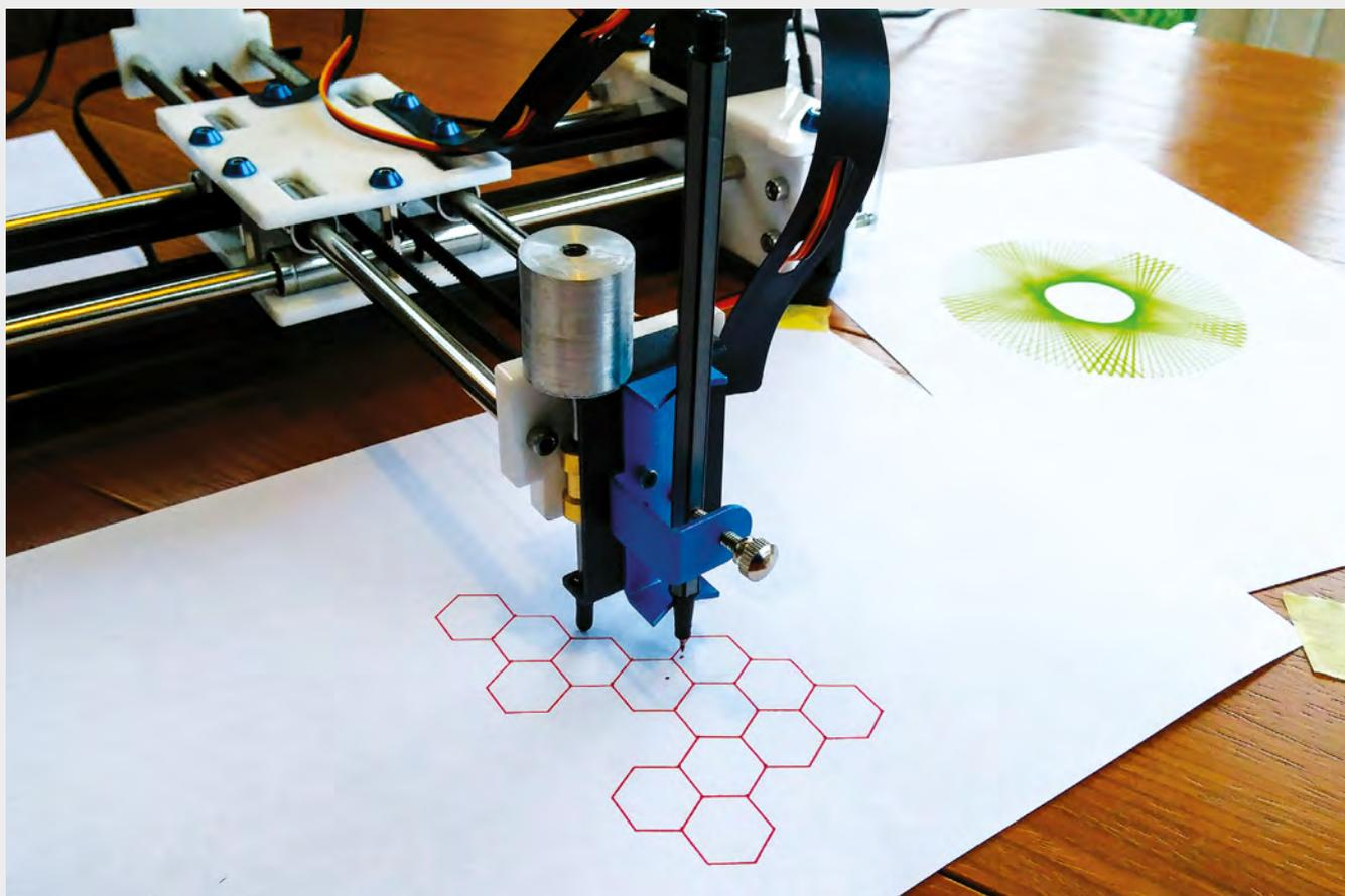
the whole range of EleksMaker products. We then turn on the machine and are nearly ready to draw something. The software is reasonably intuitive. There is a 'jog' control, allowing you to move the pen plotting head and a set home button, so you can zero the machine when it's in the desired start position.
