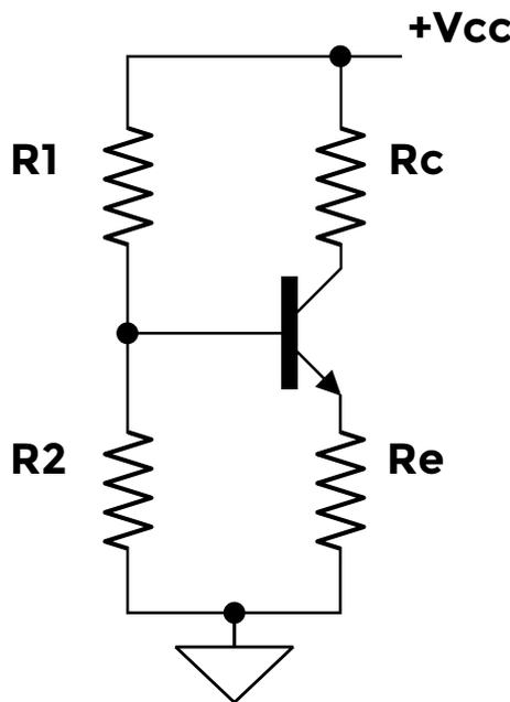
**Figure 6** ♦ Current source driving a resistor (Rc) as a load
