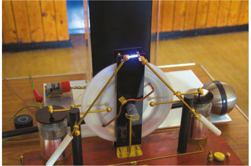
**Above** This beautiful object is a Wimshurst machine. As the disc spins, the collectors accumulate static electricity, which discharges across the spark gap
