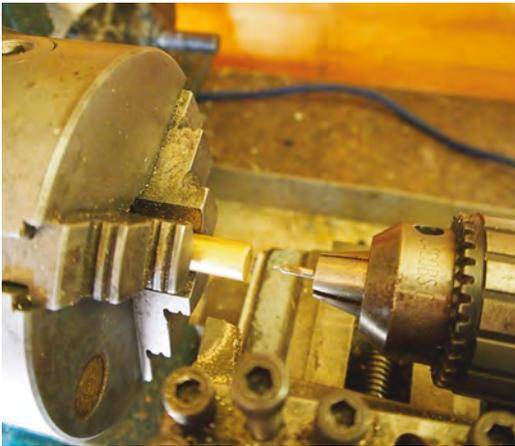
**Above** ♦ Having faced the end of the brass, we are now set up with a small centre drill in the tailstock chuck
