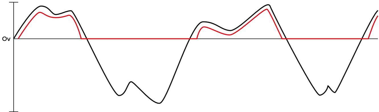
**Figure 4** ♦ The result of a positive only amplifier
