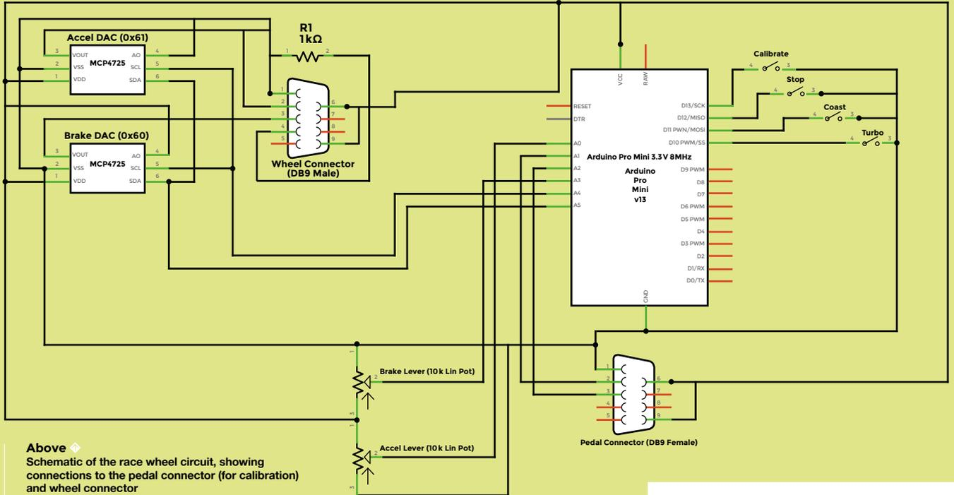
**Above** ♦ Schematic of the race wheel circuit, showing connections to the pedal connector (for calibration) and wheel connector
