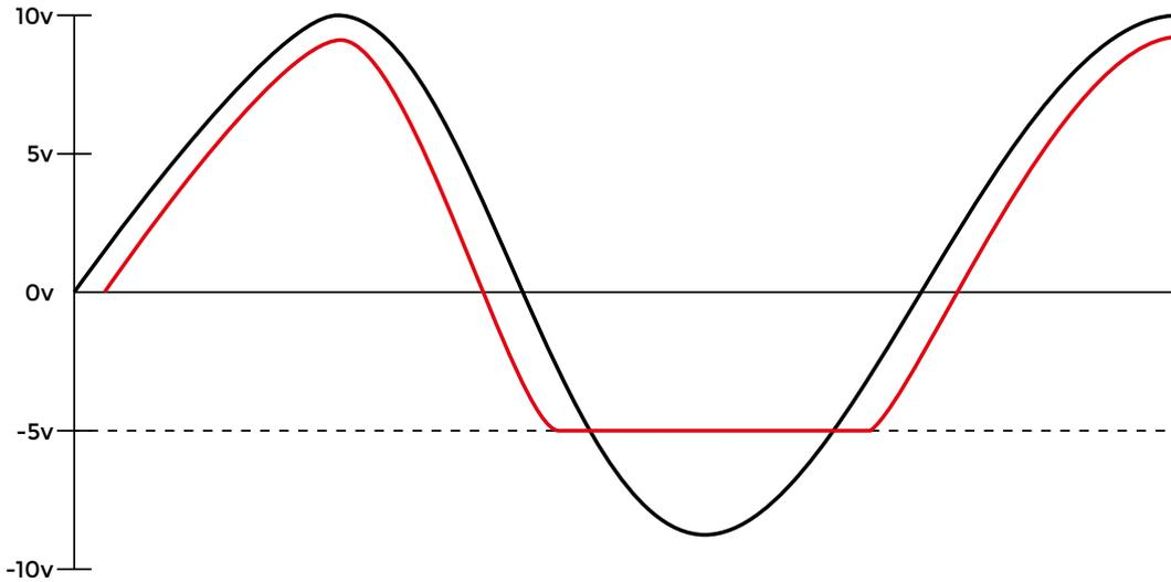
**Figure 2b** ♦ Input and clipped output of a naive emitter follower
