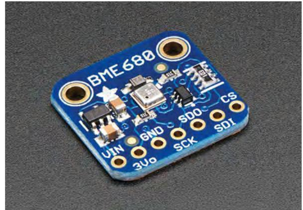
**T**he Adafruit BME680 includes a lot of environmental sensing on a tiny package. This board is able to measure temperature, humidity, barometric pressure, and VOC gases, and all over SPI or I<sup>2</sup>C, making it simple to use in almost any project.
