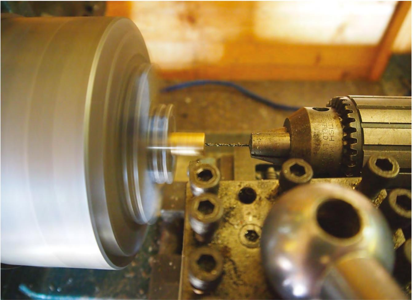
**Above** ♦ Drilling the hole that will receive the tool bits to depth
