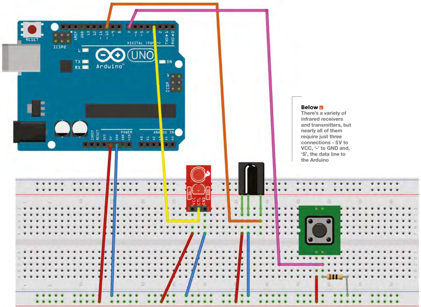
**Below** ❑ There's a variety of infrared receivers and transmitters, but nearly all of them require just three connections - 5V to VCC, '-' to GND and, 'S', the data line to the Arduino
