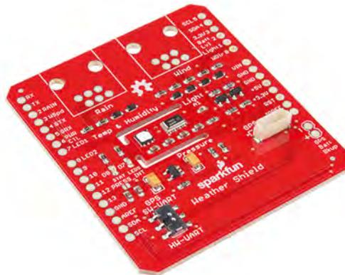
**Left** ♦ An expandable weather shield for Arduino
