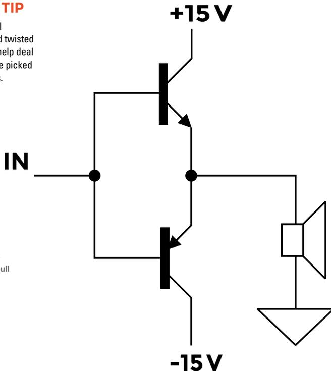
Figure 10 Basic push-pull amplifier
