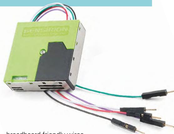
breadboard-friendly wires that are colour coded for simple hook-ups. Sensirion also provides drivers for both the UART protocol and I<sup>2</sup>C. Just keep in mind that if you plan to use this with your Arduino, it works best with UART and not I<sup>2</sup>C. As always, check out the datasheet for more information. □
