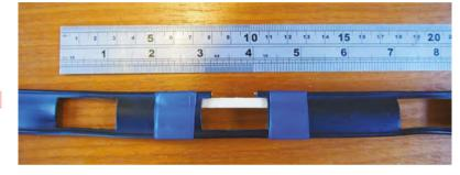
Above The gap, cut and reinforced
