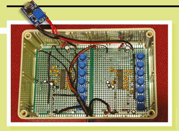
more useful point. I've found the best results (for my hearing) by selecting the following frequencies (which are approximate, bearing in mind the limited range of standard value capacitors that are easily available): 160 Hz, 345 Hz, 500 Hz, 915 Hz, 1.6 kHz, 3.4 kHz, and 6.25 kHz. These are a good balance between boosting voices while still being able to hear a reasonably full range of music.
