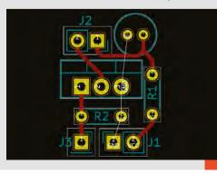
Figure 2 Importing the netlist usually results in a big messy pile of stuff getting added. Don't worry – this is correct!
