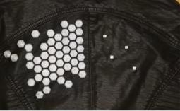
NeoPixel, then place them so that the raised square LEDs show through the square holes you made. On the back of each NeoPixel, cover each solder point with a dab of hot glue for strain relief and added protection.
