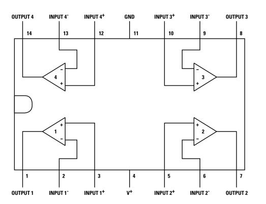
Figure 1 Functional diagram of one of the LM324N's op-amps
