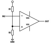
Figure 11 A basic comparator circuit
