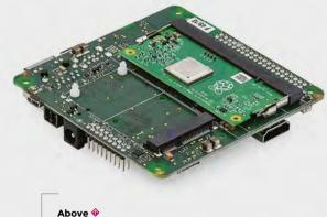
The Compute Module slots in a connector on the back of the Fin
