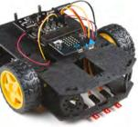
micro:bit has spawned a few interesting kits, and this kit is no exception. The SparkFun micro:bot kit leverages the micro:bit simplicity with the SparkFun moto:bit carrier board,
