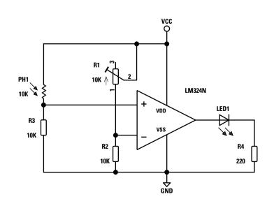
A problem with this simple comparator design shows itself when the input signal is jittering back and forth across the threshold: the output will switch back and forth between its extremes to match. For the photo comparator, this isn't an issue, but if we want to avoid that jitteriness, we need to add something.
