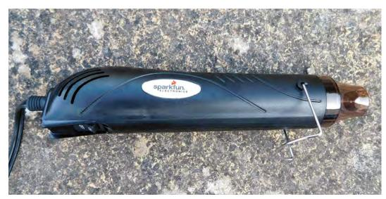
Right The SparkFun Heaterizer needs 110V, so if you're in a country with a different mains voltage, you'll need a transformer
