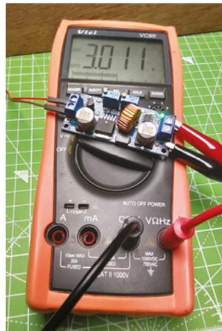
**Figure 4** ♦ Identifying which trimming potentiometer adjusts the voltage, and which adjusts the current
