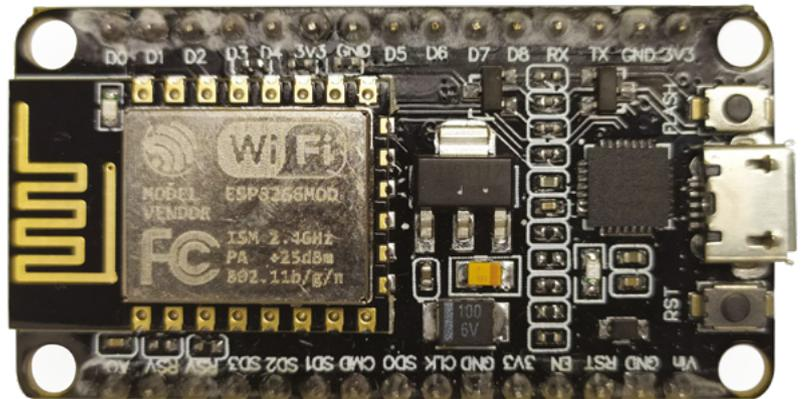
**Above** ♦ The ESP8266 comes on many different development boards. The one we've used here – the NodeMCU – is a common option, but this technique should work with others
