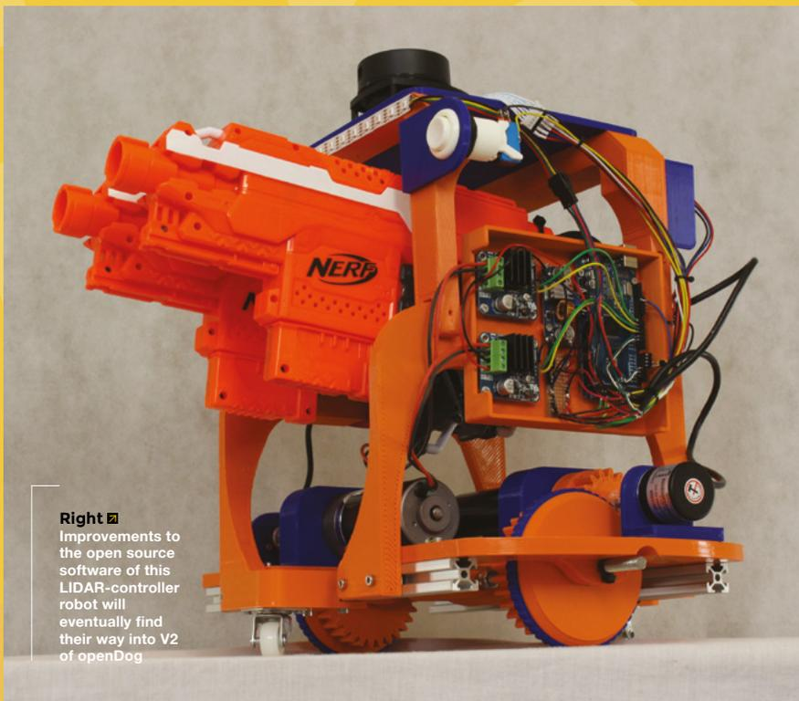
**Right** □ Improvements to the open source software of this LIDAR-controller robot will eventually find their way into V2 of openDog
