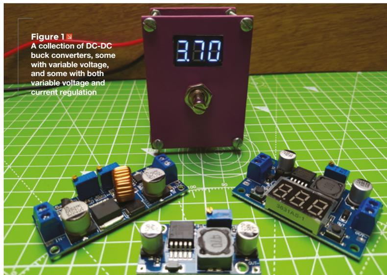
**Figure 1** A collection of DC-DC buck converters, some with variable voltage, and some with both variable voltage and current regulation
