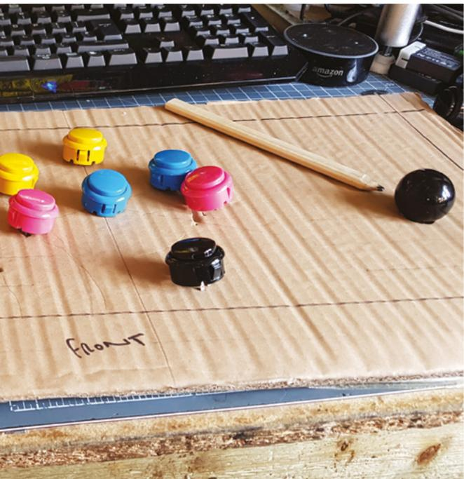
to use a cardboard template to figure out the best positioning for joysticks and switches before you drill any holes. Start with a piece of cardboard the same size as your cabinet's control console, and lay the components out on the cardboard, moving them around until they feel comfortable to use. Transfer the positions from the cardboard to the MDF control console and then cut the necessary holes.
