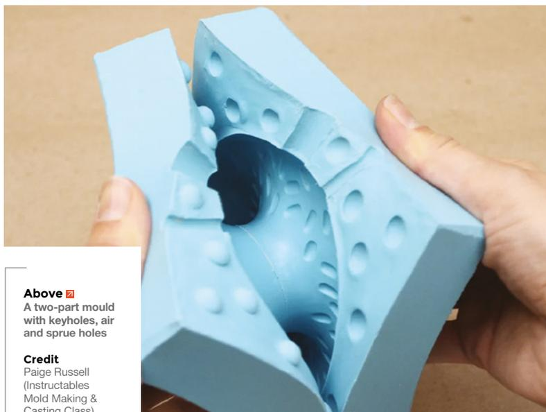
**Above** A two-part mould with keyholes, air and sprue holes
