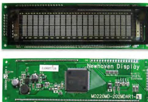
16 × 2, you can always scroll the text or make custom characters that span more than one line or section. But unlike the 16 × 2, the VFD will be much brighter, crisper, and have that cyber look that just can't be replicated any other way.
