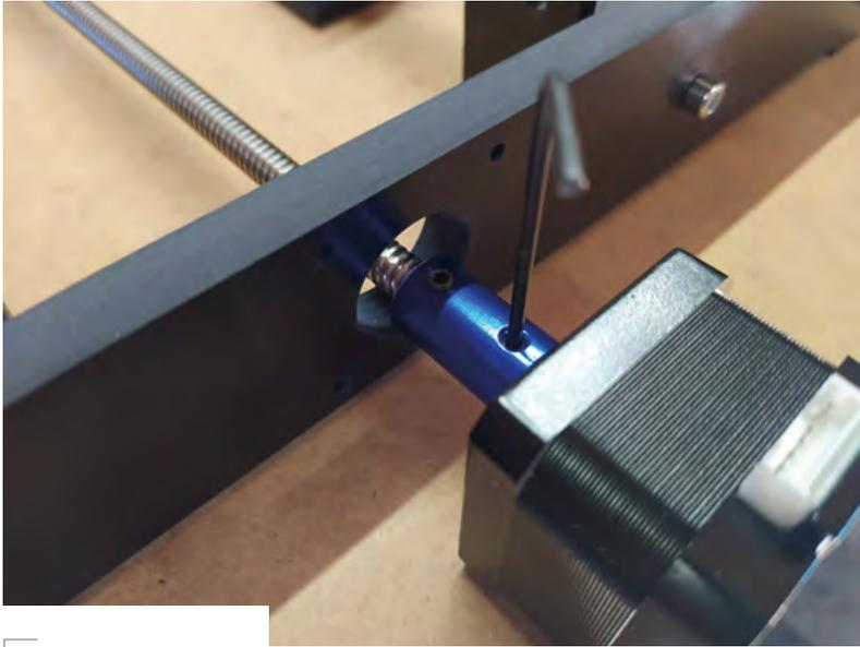
**Figure 4** ♦ Attaching the Y axis stepper motor coupler to the lead-screw and stepper motor
