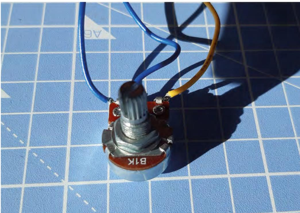
**Left** ♦ You'll find three types of potentiometers on the market: A (logarithmic); B (linear) and C (reverse logarithmic). Linear pots, like this B1K make sense for gain controls, while log pots work best for volume controls
