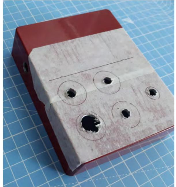
**Above** ♦ Drawing the external component layout on masking tape
