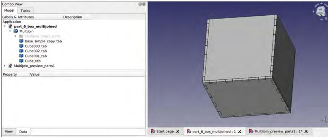
**Figure 1** ♦ Our box, complete with automatically generated interlocking tabs, and ready to be flattened and exported from the LCInterlocking workbench
