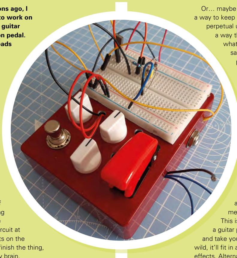
Or... maybe there was a better way... a way to keep a project in a state of perpetual unfinished-ness, but in a way that was usable. That's what I was aiming for when I sat down to build this guitar pedal tester. It's intended to be a half-way house between a breadboard and the finished pedal, with the heavy, chunky components fixed in place and connected to a breadboard, leaving me to mess with different transistors, diodes, and capacitors to make my own perfect sound. Here's how I did it.
