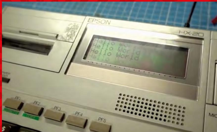
**Above** ♦ Carefully cleaning the inside of the case, and checking each connection, resulted in a largely operational 40-year-old laptop
