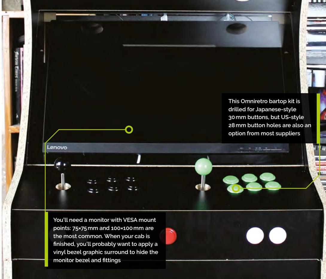
This Omniretro bartop kit is drilled for Japanese-style 30 mm buttons, but US-style 28 mm button holes are also an option from most suppliers
