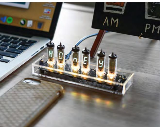
**F**luorescence by The VFD Collective on Tindie is a digital clock kit with six Soviet vacuum fluorescent display tubes that allows you to display time, or even simple messages.
