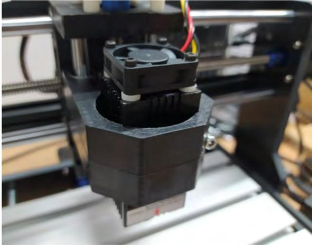
**Figure 9** ♦ The spindle mount housing has small internal corners, meaning it can snugly hold the laser module
