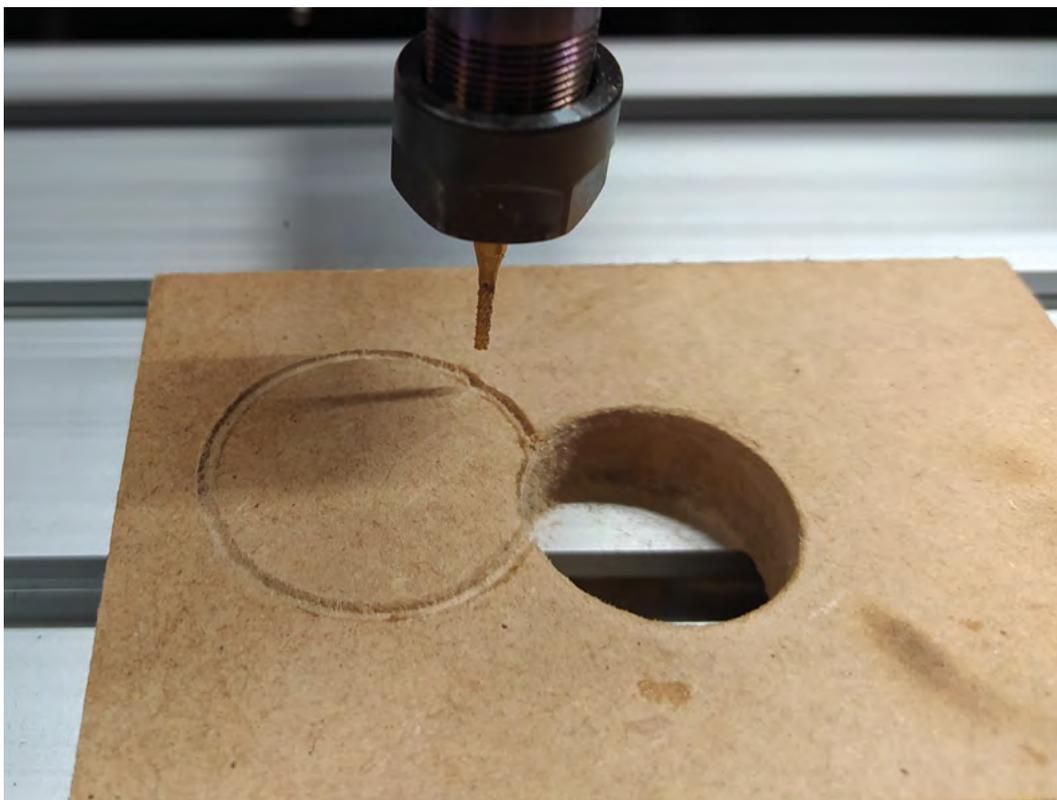
**Figure 12** ♦ After confirming our machine was working correctly with some simple jog movements and some 'air cuts', we did a tiny test cut into some scrap MDF
