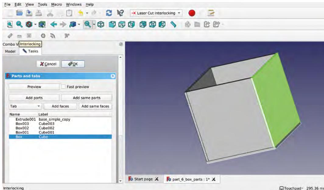
**Figure 5** Adding the parts of our box to create tabs and slots using the 'interlocking' tool
