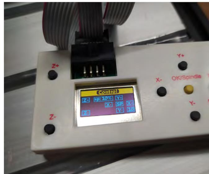
**Figure 11** ♦ The offline controller can be used to jog the machine, and also to load files to cut from an included SD card
