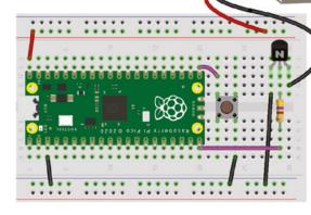
Figure 1 The wiring diagram for the quiz buzzers system
