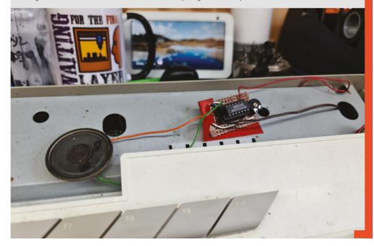
Left The Atari was hacked at some point to add a simple audio amplifier with an internal speaker, and an audio output on the rear of the case
