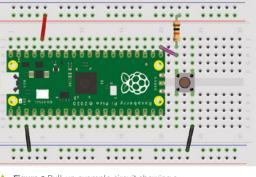
Figure 2 Pull-up example circuit showing a pull-up resistor and switch connecting to ground
