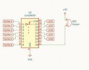
Figure 7 The schematic diagram makes it easier to see which components are wired together. To avoid crossing lines, labels have been used; labels with the same name are connected together
