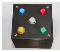
Figure 8 The finished game can be installed into an enclosure. This one is 3D-printed, but you could just use a plastic storage box and drill holes for the buttons
