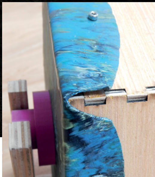
Above ⬆ PLA sheet is easy to work with hand tools. We bent this with a heat gun and snipped the corners with scissors
