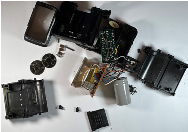
Figure 6 ♦ The grey cylinder is the capacitor that is charged up to provide a high-voltage pulse to excite the gas in the flash tube, causing a flash of light when the flash is fired
