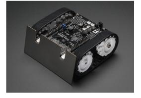
he Zumo Robot is an Arduino-based tracked robot that is less than 10 cm × 10 cm, which qualifies it for mini sumo competitions. Power is provided by two micro metal gearbox motors, and it features a stainless steel bulldozer-like blade for pushing around
