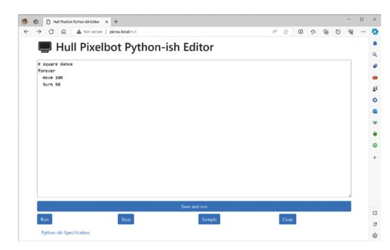
Figure 1 The program being edited makes the robot move in a square. Can you change it to make a robot move in a hexagon?
