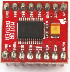
Figure 2: The motor driver is an SMD IC soldered onto a breakout board, allowing it to be used with a breadboard you can normally use a single power supply for both your Raspberry Pi and the motors.
