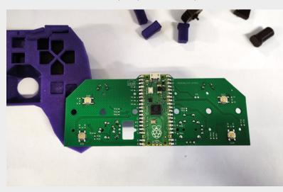
easier option of buying the base PCB that comes with one side of surface-mount components already soldered on. We also got the additional components directly from Input Labs to make sure we got the correct parts.
