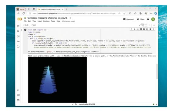
we do one of two things. Either we draw a line segment to the next point or – one out of every eleven times – it draws an extra line an additional 10 mm out of the side. Since there's nothing below this line, it will sag down against the side of the tree.
