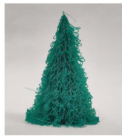
With FullControl, you build up a list of steps. Each step is generated by a FullControl method, and when you're finished, you can convert these into G-code. Our Christmas tree is:
