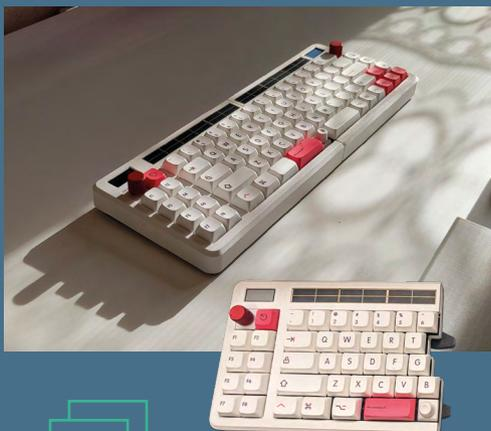
**Left** ♦ Solar panels along the top of the case trickle-charge the Aloidia keyboard
