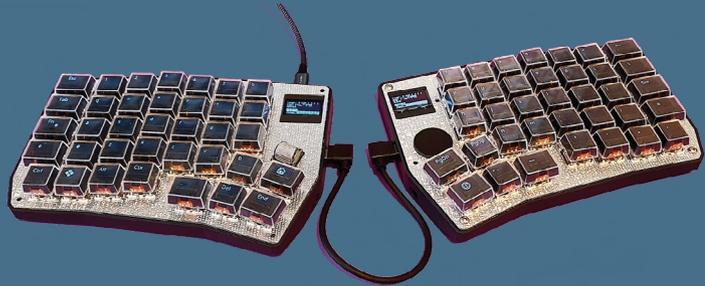
**Above** Each keycap has a tiny OLED, so can easily be relabelled if needed
