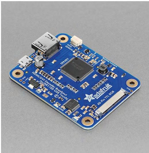
**T**he TFP401 HDMI/DVI Decoder is a small board that serves a useful purpose. Now you can easily add a 40-pin TTL/TTF display, via HDMI/DVI video, to a Raspberry Pi project.
