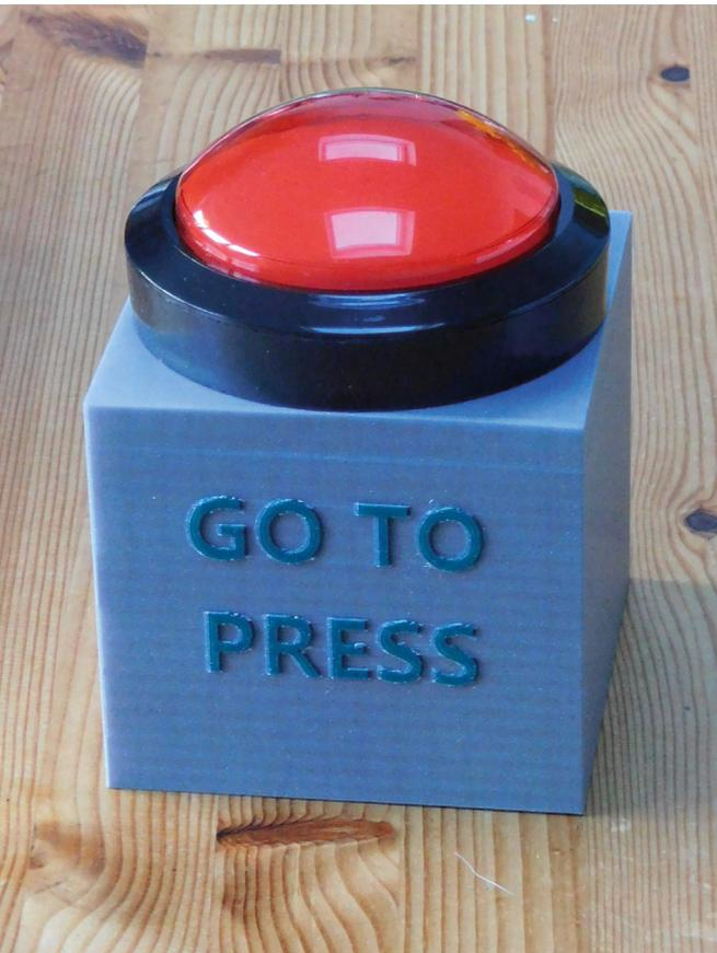
or VBUS, but we thought we'd keep the option for adding light effects in the future). The LED has a built-in resistor, so we can just connect it up directly to pin 0 and ground. The LED pins are on either side of the switch (see **Figure 1**). You can use either one as ground and power, and then just turn the LED around to match.
