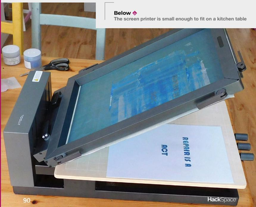
Screen printing has been around for a long time. The basic idea is that you have a fine mesh of fabric. You cover most of this mesh with some sort of impermeable barrier, but the bit where you want ink (or paint) to get through, you leave uncovered. You then hold this screen against the thing you want to print onto and squeegee the ink (or paint) through it. If all goes well, you should have a perfect replica of your design on the surface below.
