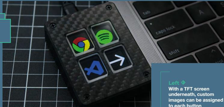
Left ♦ With a TFT screen underneath, custom images can be assigned to each button
