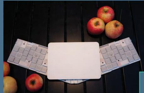
**S**eeking a better portable keyboard for his coffee shop visits, Sergei Silnov set about crafting the 'perfect keyboard' with a folding mechanism and comfortable typing action. A central 3D-printed hinge enables the two keyboard halves to fold up into a rectangular portable package with 2cm thickness. When unfolded, a central kickstand can be lifted up to hold a phone; or the two halves can be pulled further apart to accommodate an Apple Magic Trackpad, attached magnetically.
