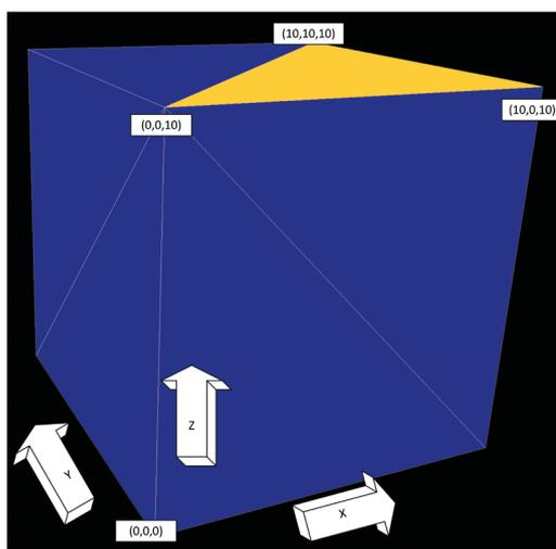
well. In the case of our pirate coordinate system, the X axis is on the vector (1, 0, 0) and the Y axis is on the vector (0, 1, 0).
