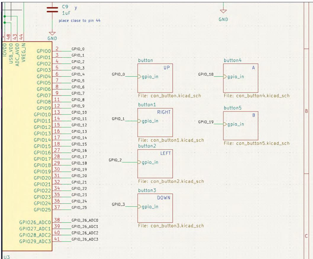
To add the buttons to our schematic, we created a custom 4-pin schematic symbol and inserted it into a hierarchical sheet. We wired the GPIO pin and the other pins to ground and then brought out the GPIO hierarchical pin. We then copied the hierarchical sheet to create six versions, one for each button, adjusting the label and the sheet name as we added each (Figure 2). Again, we've covered this in earlier sections.
