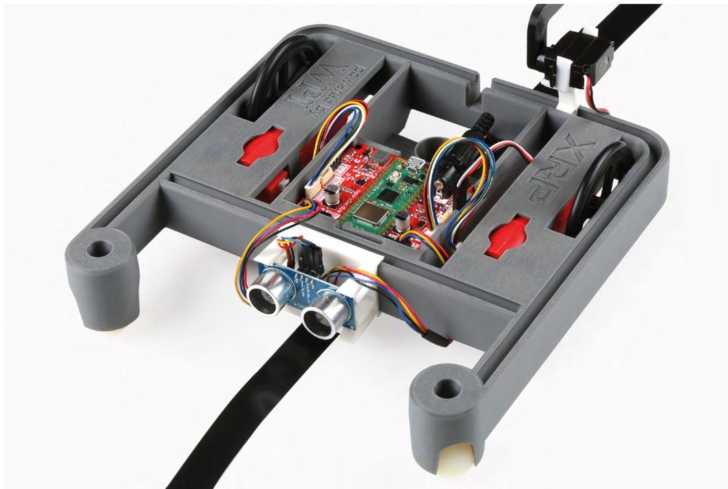
**S**parkFun has a new board with loads of potential called the **Experiential Robotics Platform (XRP)**. It's designed to allow for easy hardware and software iterations of robots thanks to its compatibility with Blockly, Python, and the FIRST Robotics coding development tool. At the core of the XRP board is Raspberry Pi Pico W, enabling seamless wireless LAN and Bluetooth connectivity, as well as a familiar GPIO interface.
