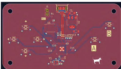
Having ordered the boards, one final fun activity on the hardware side of this build was to export a STEP file from KiCad to model around in FreeCAD. To export a basic STEP file from the KiCad PCB Editor, select File > Export and then choose STEP as the output format. Note that we haven't added custom 3D models for all of our custom components, so obviously the STEP file isn't completely correct, but it serves as a good enough guide to model around in FreeCAD. →
