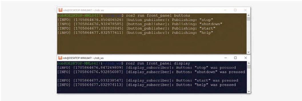
**Figure 6** These packages are running on a PC under the Windows Subsystem for Linux, but they could just as easily be running on a Raspberry Pi
