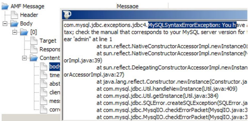
Figure 13 – Stack trace showing injection.
