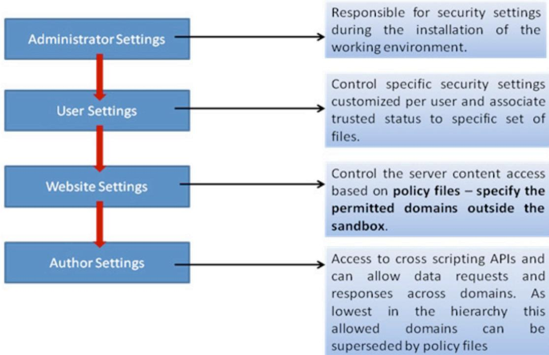
Figure 5 – Summarizing the Stakeholder Concept of the Flash Security Model.
