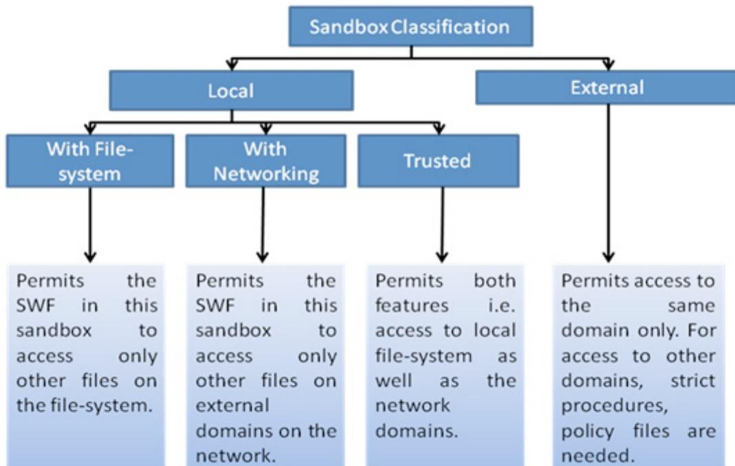
Figure 6 – Synopsis of the Sandbox Model of Flash Security.
