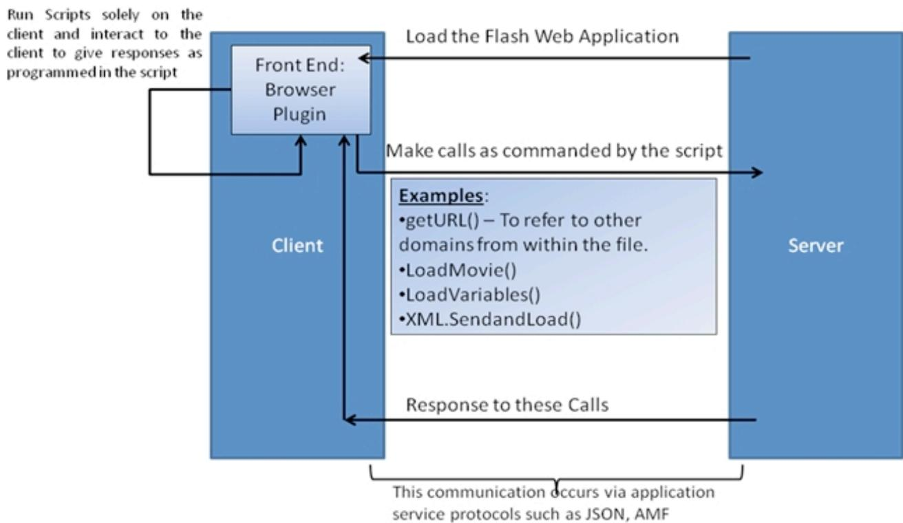
Figure 4 – Communication within Flash based RIA
