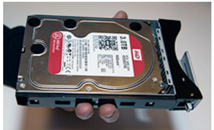
The HDD enclosures can hold 3.5" or 2.5" disks and are quite sturdy, with rubber pads
