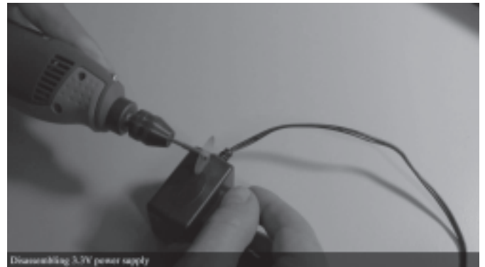
Disassembling 3.3V power supply
