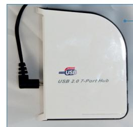
**Powered hub:** A USB 2 powered hub is essential for anything you do with the Raspberry Pi.
