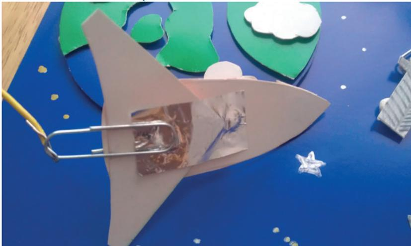
Our rocket is really a hidden link to the Raspberry Pi GPIO ground pin, which when connected to a pin that is high will pull that pin low, changing its state.
