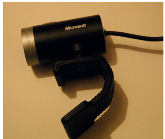
Our webcam is a Microsoft LifeCam HD, which has a maximum resolution of 1280 x 720, but we set the resolution to its lowest to gain more speed.
