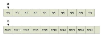
**Above** Array elements are stored sequentially in memory, with the array name a pointer to the first element. Multi-dimensional array elements are stored with the elements with neighbouring values, in the rightmost index next to each other
