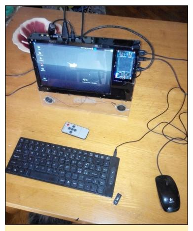
The finished laptop case, with speakers installed at the bottom of the clear plexiglass front, a handy I/O shield for quick hardware prototyping, and a beautiful IO.I" HD monitor
