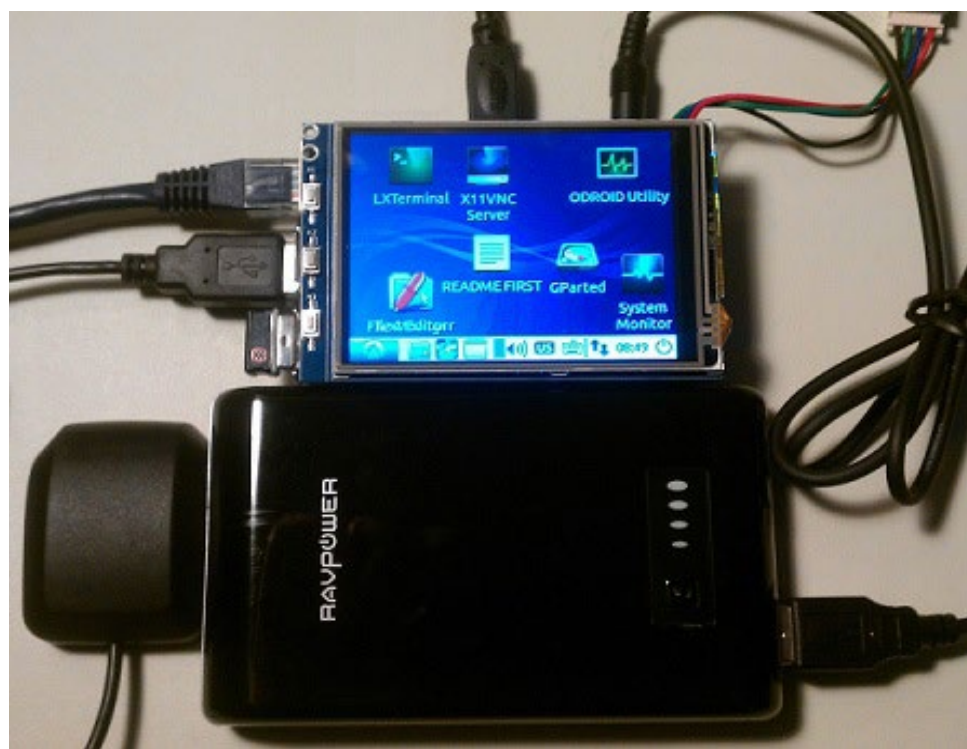
Figure 1: ODROID-C1, GPS, touchscreen and battery setup
