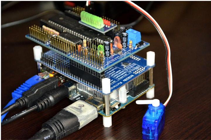
**24 channel Data Acquisition project using 3 GPIO, de-multiplexer and 1 SPI chip select**
