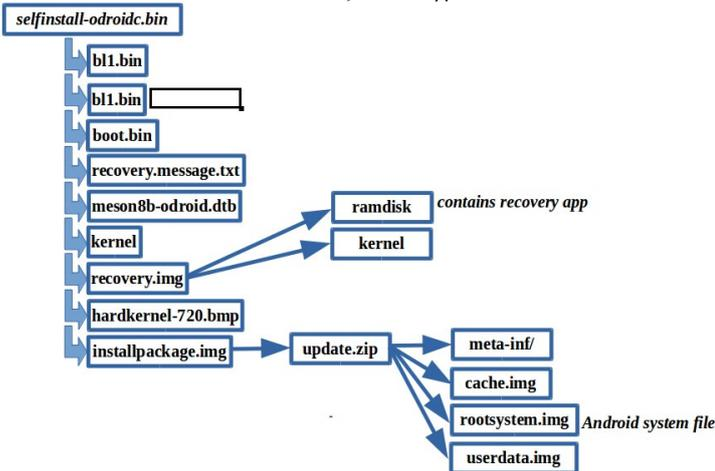
Figure 1: Content of selfinstall-odroidc.bin
