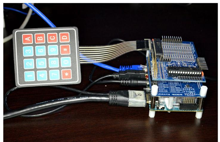
**4x4 matrix keyboard interface project using I2C I/O expanders**
