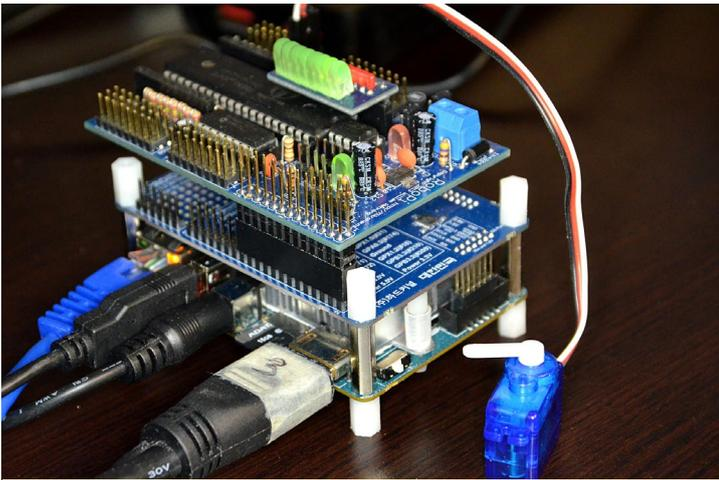
**RoboPi being tested on the ODROID-XU4 for an XU4 review**
